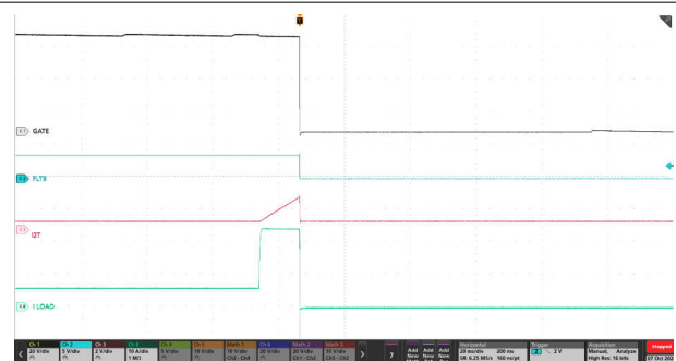
Figure 9-9. \text{I}^2\text{T} based Overcurrent Response of TPS4812-Q1 EVM for 6A to 23A Load Step
