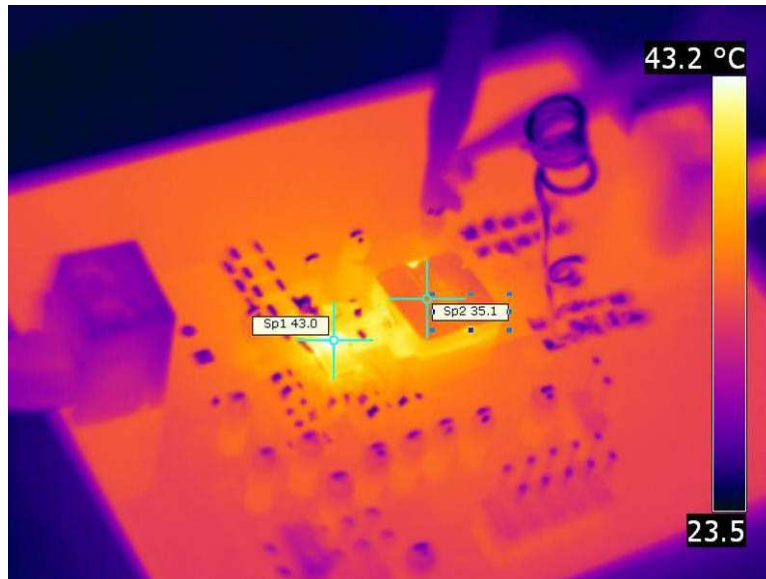
Figure 57. SP1: 43°C (TPS53515), SP2: 35.1°C (Inductor)
