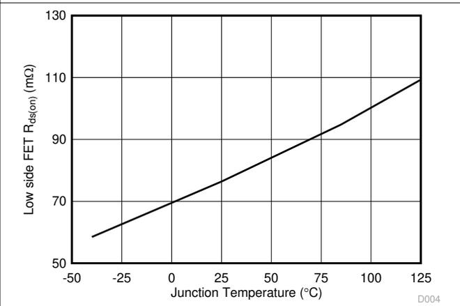
**Figure 6-4. Low-Side FET On Resistance vs Junction Temperature**
