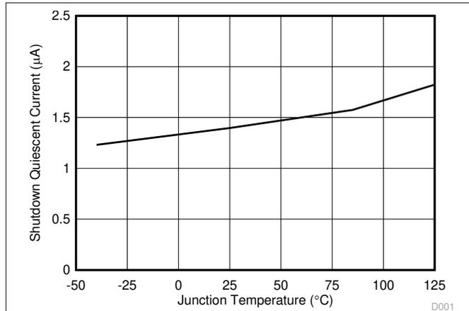
**Figure 6-1. Shutdown Quiescent Current vs Junction Temperature**
