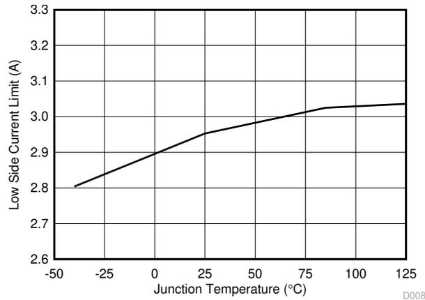
**Figure 6-8. Low-Side Current Limit Threshold vs Junction Temperature**
