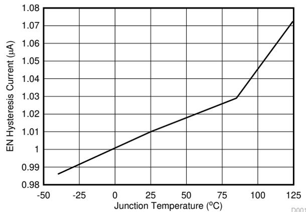
**Figure 6-12. EN Hysteresis Current vs Junction Temperature**
