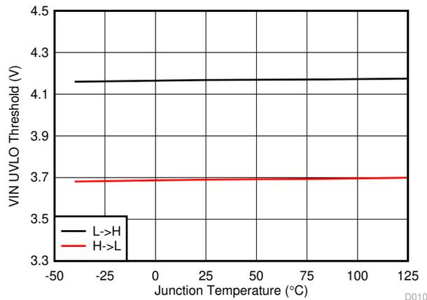
**Figure 6-10. VIN UVLO Threshold vs Junction Temperature**
