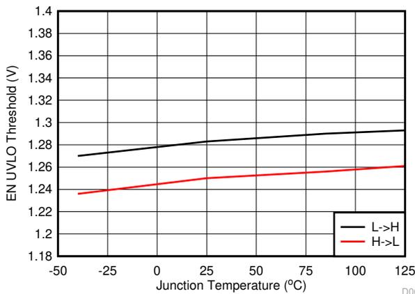
**Figure 6-11. EN UVLO Threshold vs Junction Temperature**
