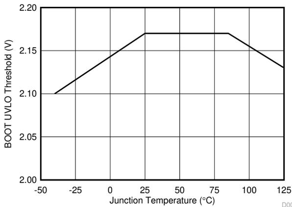
**Figure 6-9. BOOT-SW UVLO Threshold vs Junction Temperature**
