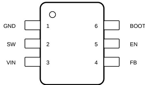
**Figure 5-1. 6-Pin SOT-23 DDC Package (Top View)**
