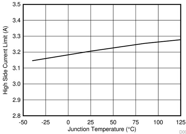
**Figure 6-7. High-Side Current Limit Threshold vs Junction Temperature**
