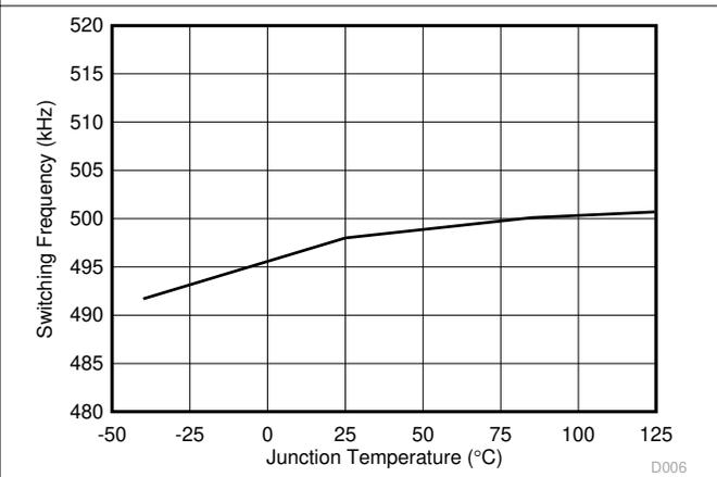
**Figure 6-6. Centre Switching Frequency vs Junction Temperature**
