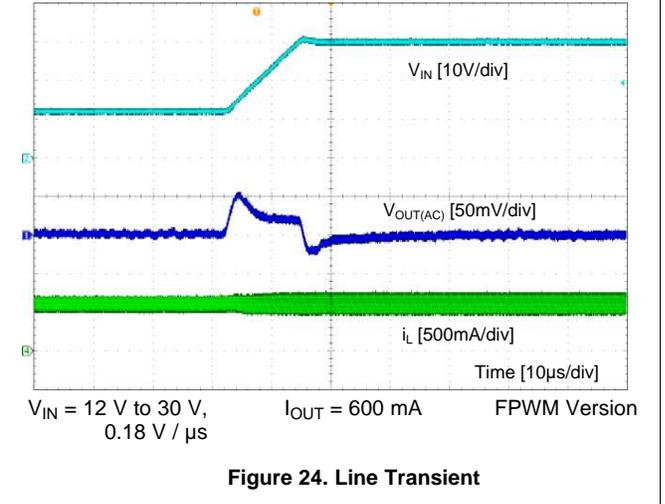
Unless otherwise specified the following conditions apply:  $V_{IN} = 12\text{ V}$ ,  $V_{OUT} = 5\text{ V}$ ,  $f_{SW} = 1.1\text{ MHz}$ ,  $L = 18\text{ }\mu\text{H}$ ,  $C_{OUT} = 22\text{ }\mu\text{F}$ ,  $T_A = 25\text{ }^\circ\text{C}$
