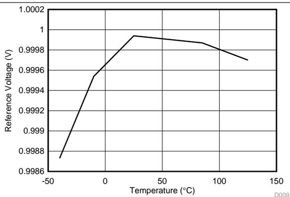
Figure 11. Reference Voltage vs Temperature
