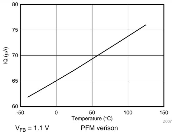
Figure 9.  $I_Q$  vs Temperature
