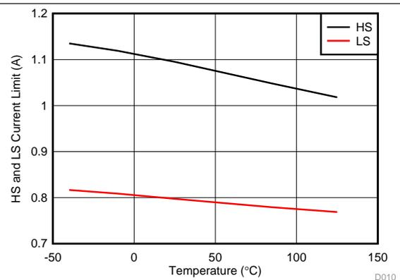
Figure 12. HS and LS Current Limit vs Temperature
