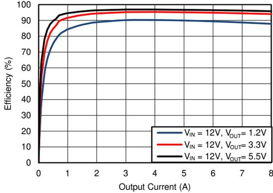
**Figure 6-13. Efficiency, Mode = FCCM,  $F_{SW} = 400\text{kHz}$**
