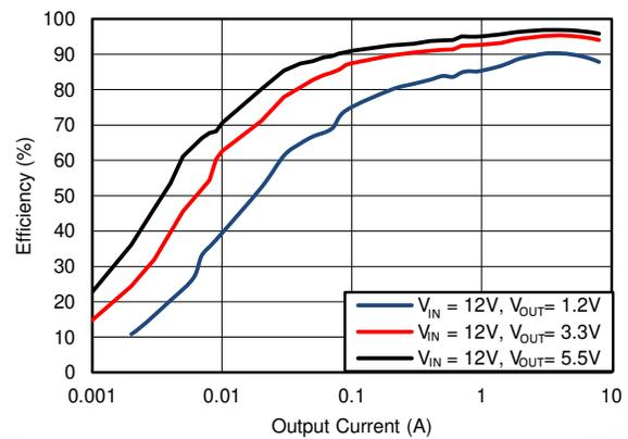
Figure 6-12. Efficiency, Mode = DCM, F<sub>SW</sub> = 400kHz
