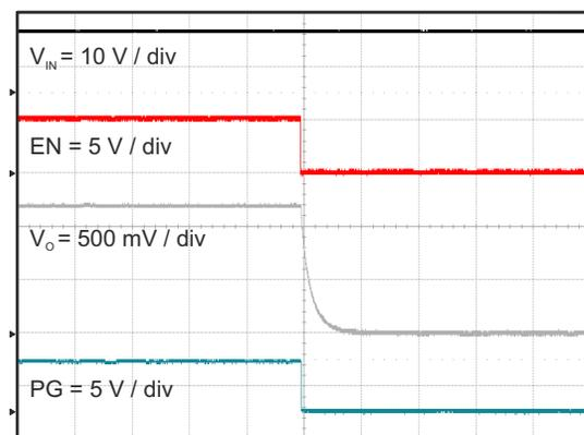
**Figure 8-17. Shut Down Relative to EN Falling**
