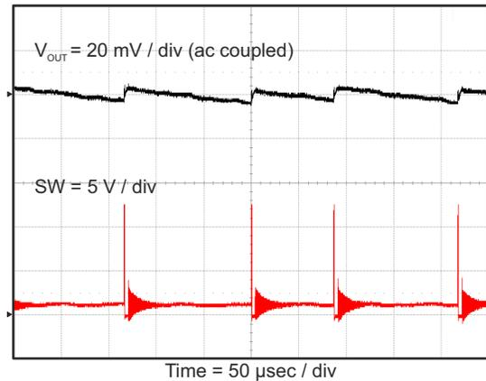
**Figure 8-11. Output Voltage Ripple,  $I_{OUT} = 10 \text{ mA}$**
