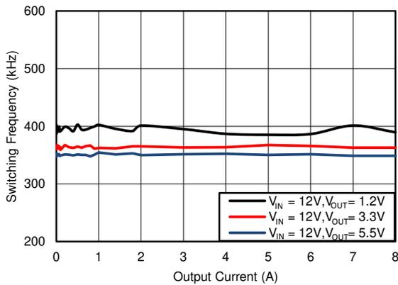
**Figure 6-17.  $F_{SW}$  Load Regulation, Mode = FCCM,  $F_{SW} = 400\text{kHz}$**
