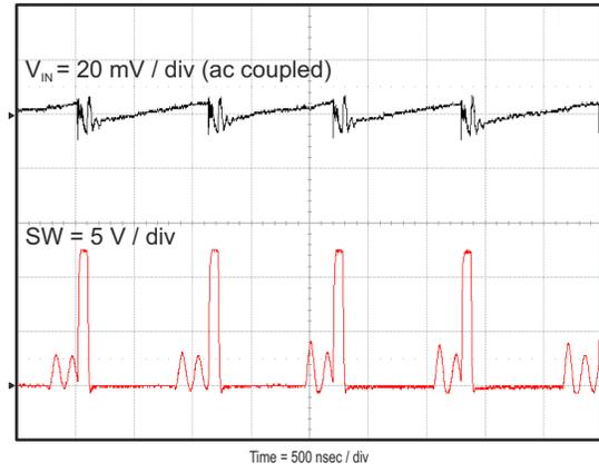
**Figure 8-9. Input Voltage Ripple,  $I_{OUT} = 700 \text{ mA}$**
