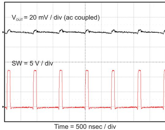
**Figure 8-13. Output Voltage Ripple,  $I_{OUT} = 8 \text{ A}$**
