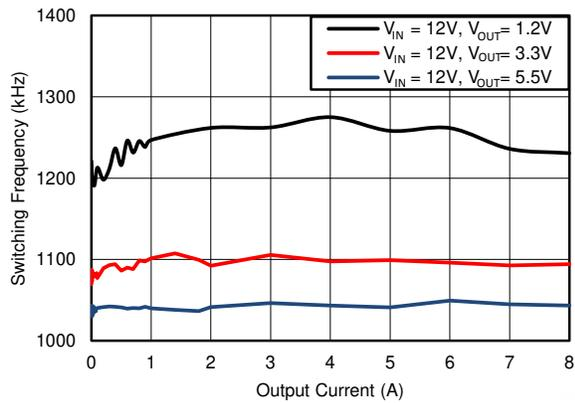
**Figure 6-19.  $F_{SW}$  Load Regulation, Mode = FCCM,  $F_{SW} = 1200kHz$**
