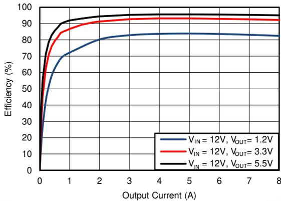
**Figure 6-15. Efficiency, Mode = FCCM,  $F_{SW} = 1200\text{kHz}$**
