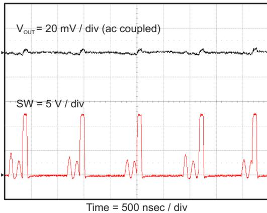
**Figure 8-12. Output Voltage Ripple,  $I_{OUT} = 700 \text{ mA}$**
