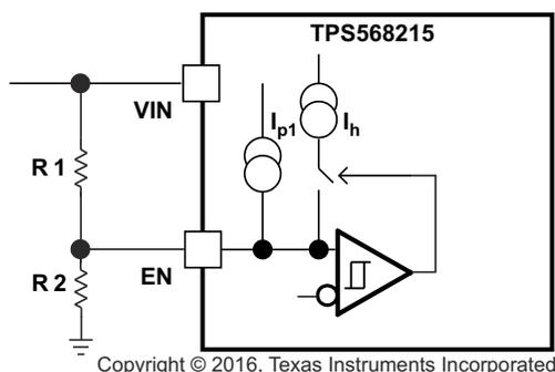
**Figure 7-2. Adjustable VIN Under Voltage Lock Out**
