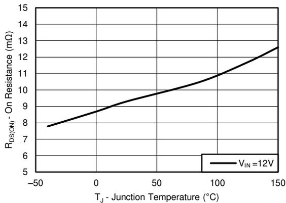
Figure 6-5. Low-side R<sub>ds(on)</sub> vs Temperature
