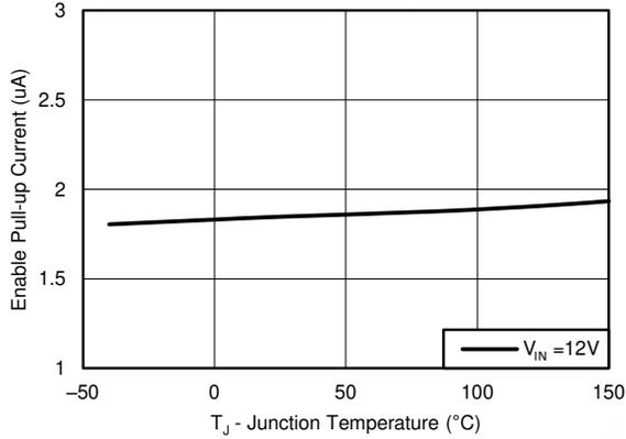
Figure 6-7. Enable Pull-Up Current, V<sub>EN</sub> = 1.0V
