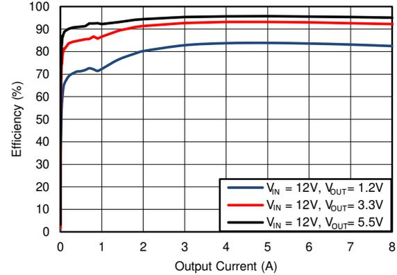
**Figure 6-14. Efficiency, Mode = DCM,  $F_{SW} = 1200\text{kHz}$**
