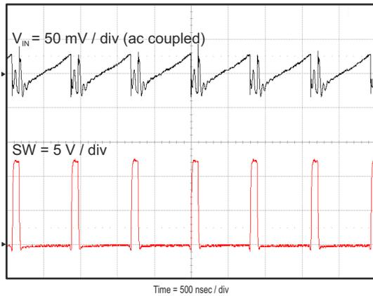
**Figure 8-10. Input Voltage Ripple,  $I_{OUT} = 8 \text{ A}$**
