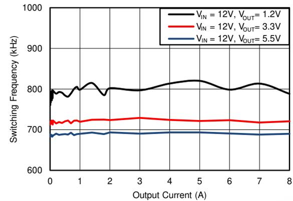
**Figure 6-18.  $F_{SW}$  Load Regulation, Mode = FCCM,  $F_{SW} = 800\text{kHz}$**
