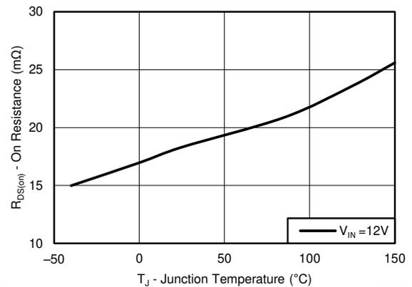
Figure 6-4. High-side R<sub>ds(on)</sub> vs Temperature
