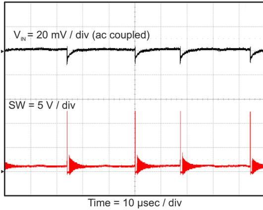
**Figure 8-8. Input Voltage Ripple,  $I_{OUT} = 10 \text{ mA}$**
