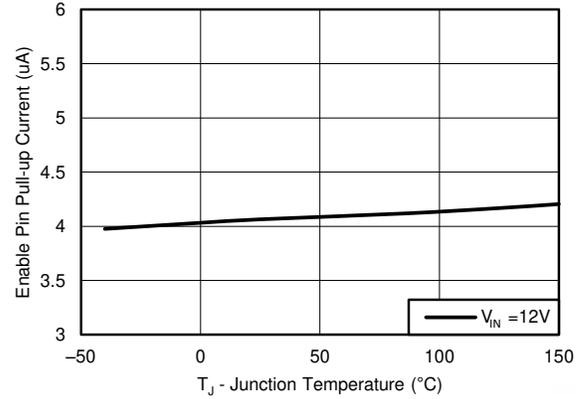
Figure 6-8. Enable Pull-Up Current, V<sub>EN</sub> = 1.3V
