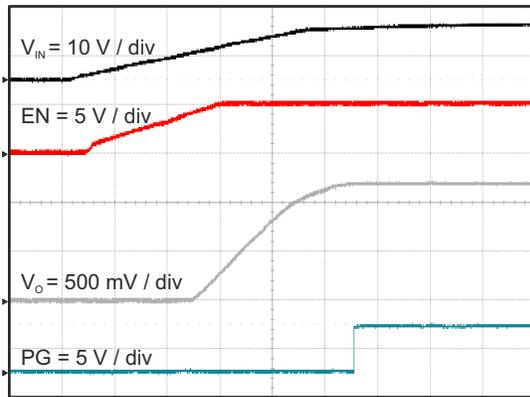
**Figure 8-14. Start Up Relative to  $V_{IN}$  Rising**
