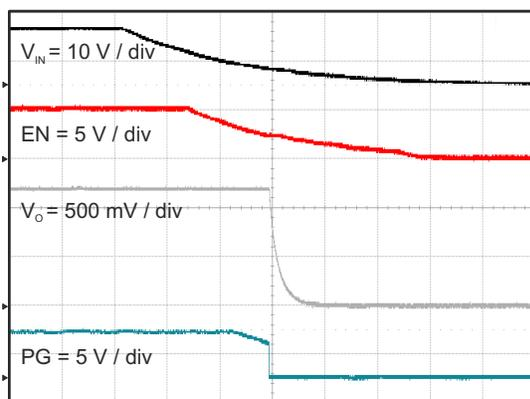
**Figure 8-16. Shut Down Relative to  $V_{IN}$  Falling**
