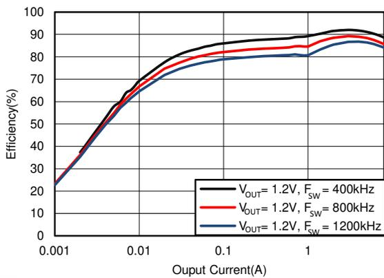
Figure 6-11. Efficiency with Internal VREG5 = 4.7 V, V<sub>IN</sub> = 12 V
