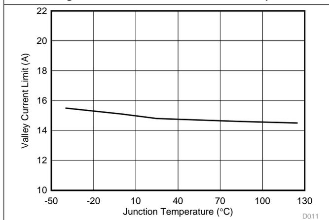
Figure 11. Valley Current Limit vs Junction Temperature
