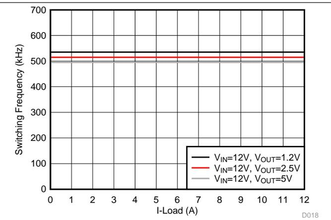
Figure 16. Switching Frequency vs Load Current, FCCM
