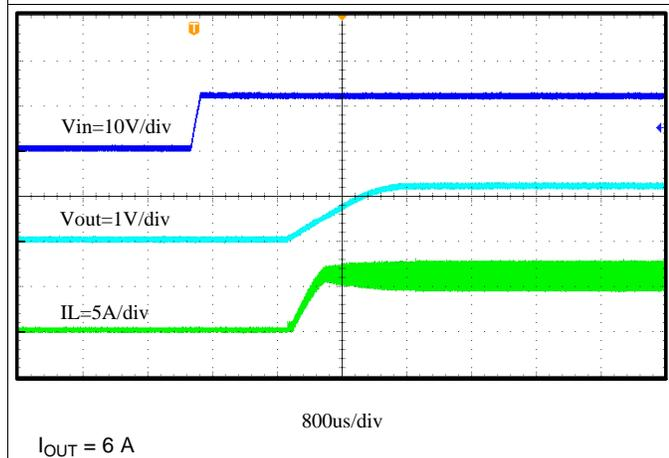
Figure 27. Start Up Relative to V<sub>IN</sub> Rising
