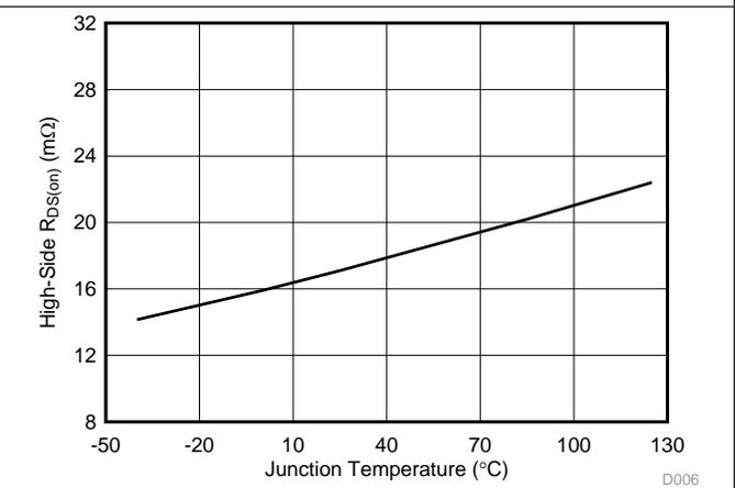
Figure 6. High-Side R<sub>DS(on)</sub> vs Junction Temperature
