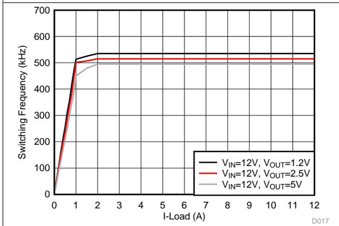
Figure 15. Switching Frequency vs Load Current, Eco-mode
