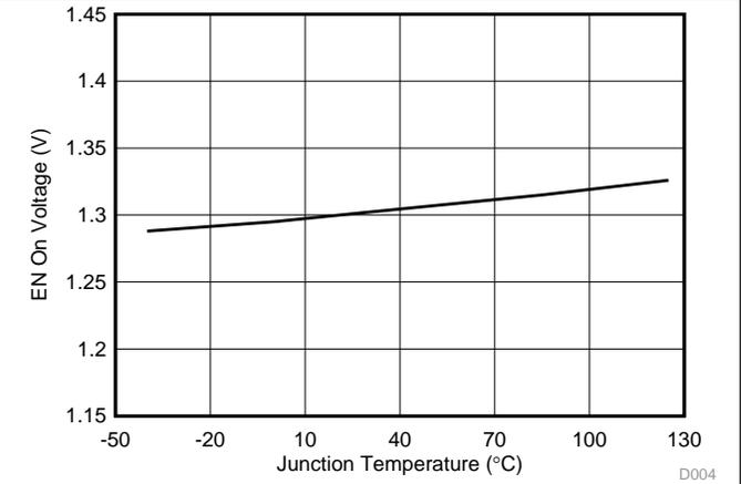
Figure 4. Enable On Voltage vs Junction Temperature
