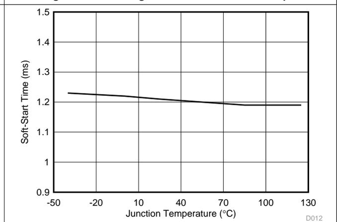
Figure 12. Soft-Start Time vs Junction Temperature
