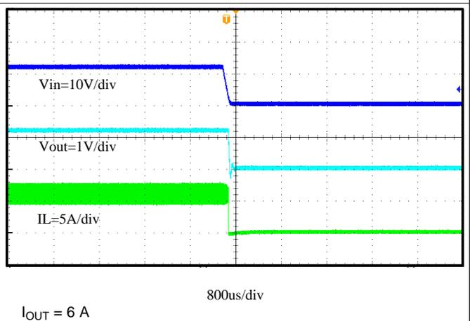
Figure 28. Shut Down Relative to V<sub>IN</sub> Falling
