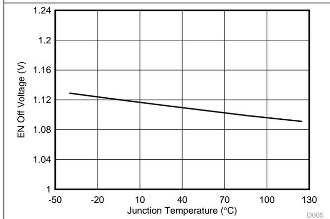
Figure 5. Enable Off Voltage vs Junction Temperature
