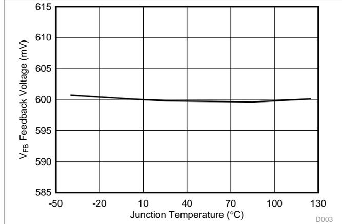
Figure 3. Feedback Voltage vs Junction Temperature
