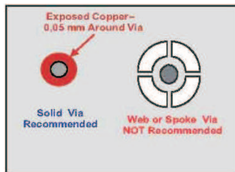
Figure 27. Thermal Via Connection at the Bottom Layer
