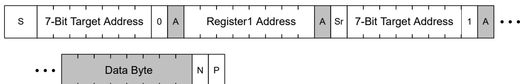
Figure 7-15. I 2 C Write Data Format
