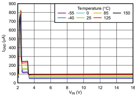
Figure 5-17. TPS76933 Ground Current vs Input Supply (New Chip)
