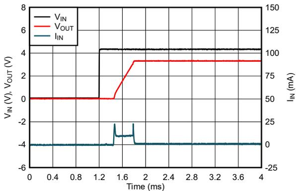
Figure 5-35. LDO Start-Up Time With Input Supply (New Chip)
