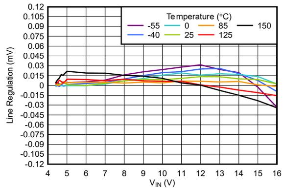
Figure 5-10. TPS76933 Line Regulation vs Free-Air Temperature (New Chip)
