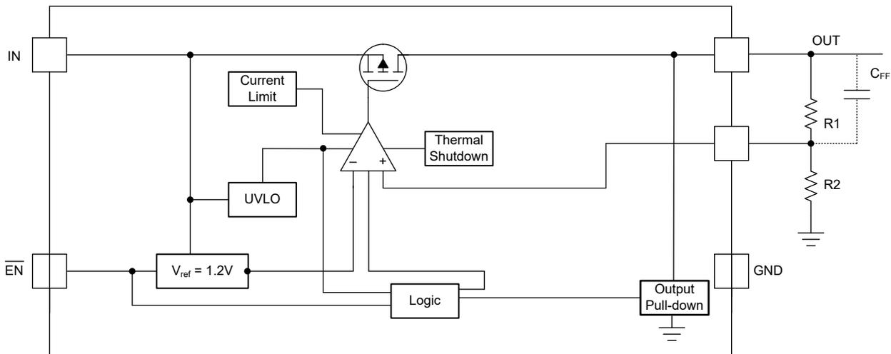
Figure 6-3. TPS76901 Adjustable Functional Block Diagram (New Chip)
