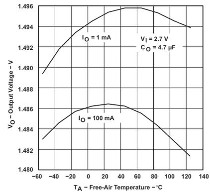
**Figure 5-6. TPS76915 Output Voltage vs Free-Air Temperature (Legacy Chip)**
