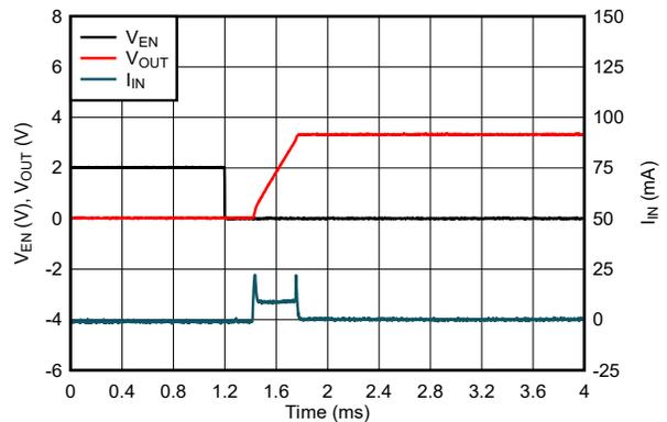
Figure 5-36. LDO Start-Up Time With EN (New Chip)
