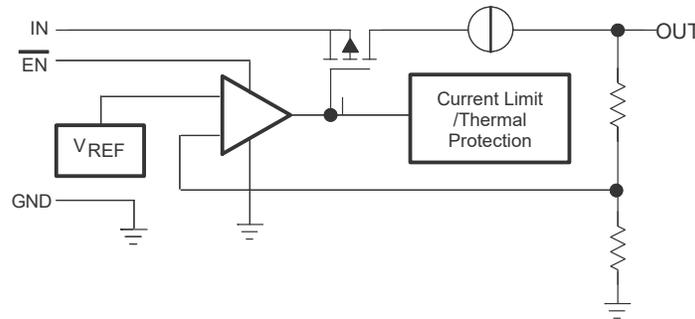
Figure 6-2. TPS769 Functional Block Diagram (Legacy Chip)
