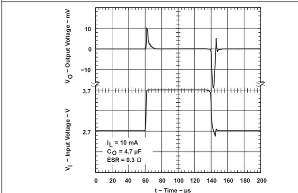
**Figure 7-8. TPS76915 Line Transient Response (Legacy Chip)**
