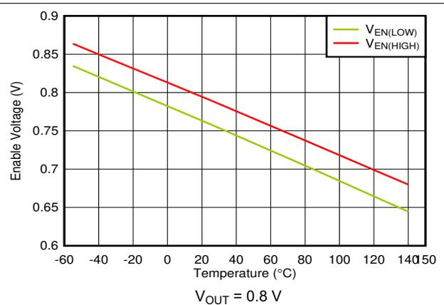
Figure 6-38. EN High and Low Threshold vs Temperature
