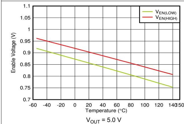
Figure 6-39. EN High and Low Threshold vs Temperature
