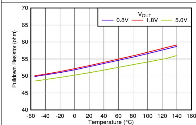
Figure 6-41. Pulldown Resistor vs Temperature and  $V_{OUT}$
