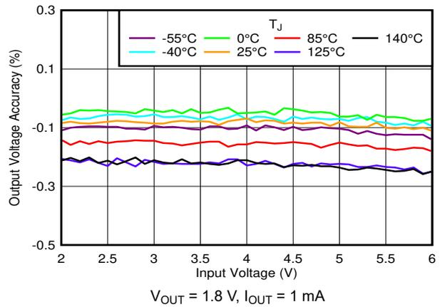
Figure 6-26. Output Accuracy vs  $V_{IN}$  and Temperature
