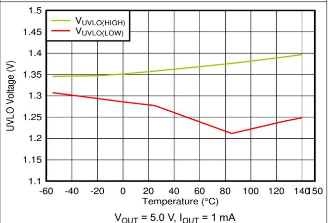
Figure 6-40. UVLO Rising and Falling Threshold vs Temperature
