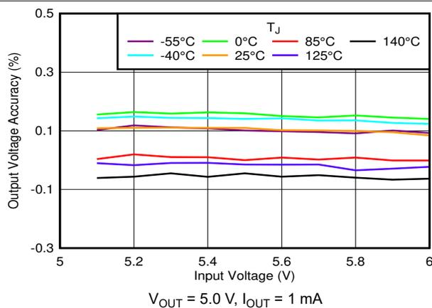
Figure 6-29. Output Accuracy vs  $V_{IN}$  and Temperature
