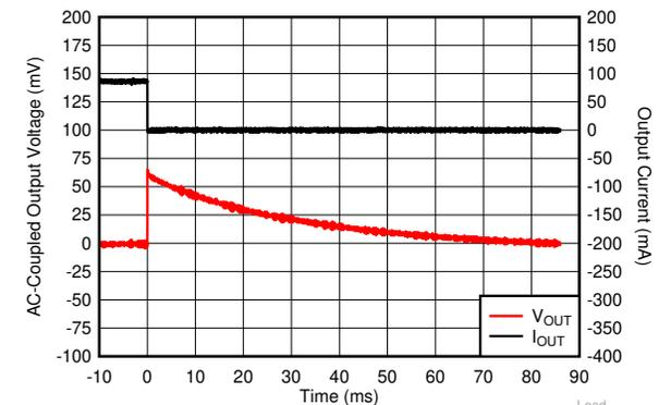
$V_{OUT} = 1.8\text{ V}$ ,  $V_{IN} = 2.8\text{ V}$ ,  $C_{OUT} = 1\ \mu\text{F}$ ,  $t_r = t_f = 1\ \mu\text{s}$
