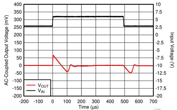
$V_{OUT} = 1.8\text{ V}$ ,  $I_{OUT} = 1\text{ mA}$ ,  $C_{OUT} = 1\text{ }\mu\text{F}$ , slew rate =  $1\text{ V}/\mu\text{s}$
