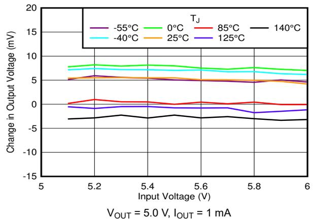
Figure 6-28. Line Regulation vs  $V_{IN}$  and Temperature
