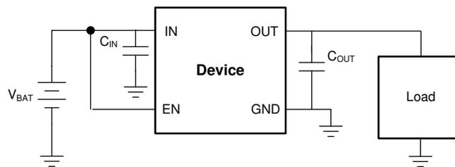
**Figure 8-4. Operation From a Battery Input Supply**
