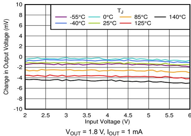
Figure 6-25. Line Regulation vs  $V_{IN}$  and Temperature
