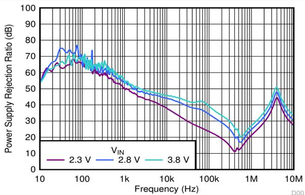
Figure 6-47. PSRR vs Frequency and  $V_{IN}$
