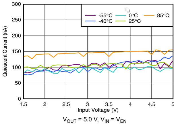
Figure 6-7.  $I_Q$  in Dropout vs  $V_{IN}$  and Temperature
