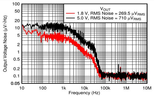
Figure 6-48. Output Noise vs Frequency and  $V_{OUT}$
