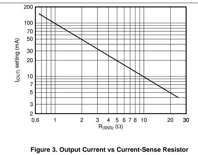
Figure 3. Output Current vs Current-Sense Resistor
