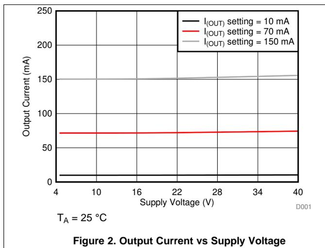
Figure 2. Output Current vs Supply Voltage
