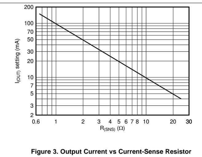
Figure 3. Output Current vs Current-Sense Resistor
