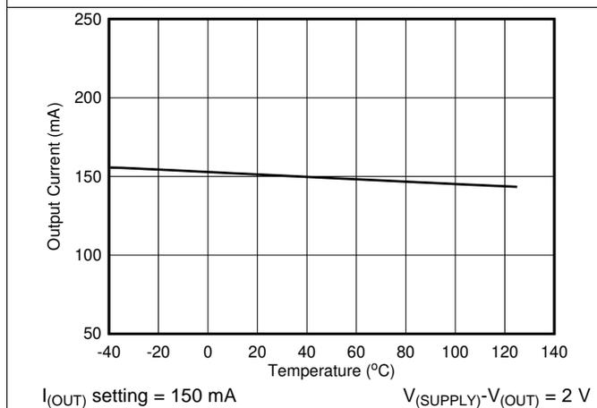
Figure 6. Output Current vs Temperature
