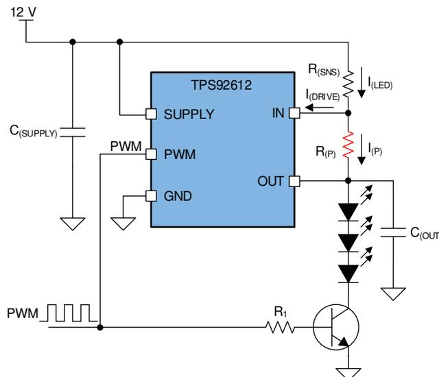
**Figure 16. PWM Control With Heat Sharing Resistor**
