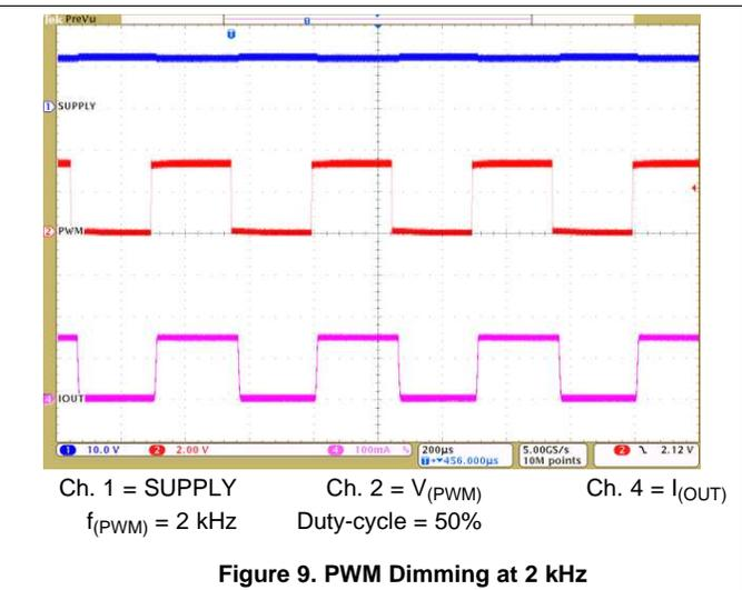
Figure 9. PWM Dimming at 2 kHz
