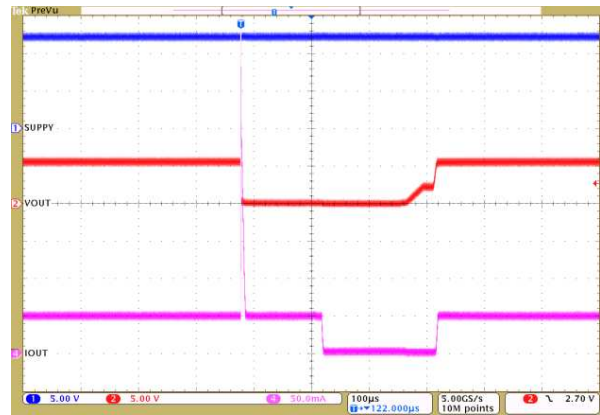
Figure 11. LED Short-Circuit Protection and Recovery
