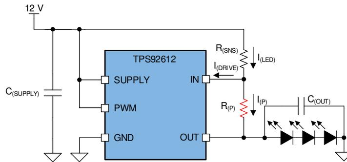
Figure 15. Heat Sharing With a Parallel Resistor
