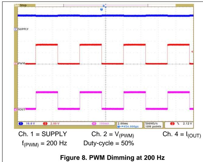
Figure 8. PWM Dimming at 200 Hz
