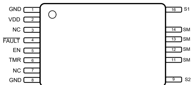
Figure 5-1. TPSI88xx DFP Package, 14-Pin SOIC (Top View)
