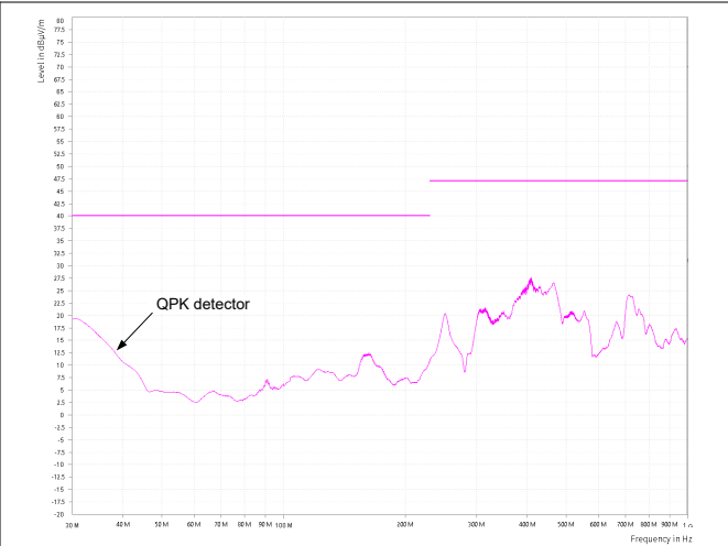
Figure 9-9. CISPR 32 Class B Radiated Emissions: Vertical Polarization
