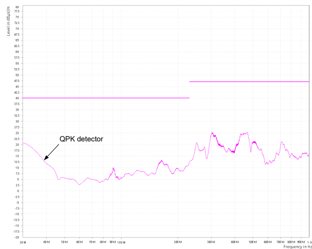
Figure 9-10. CISPR 32 Class B Radiated Emissions: Horizontal Polarization
