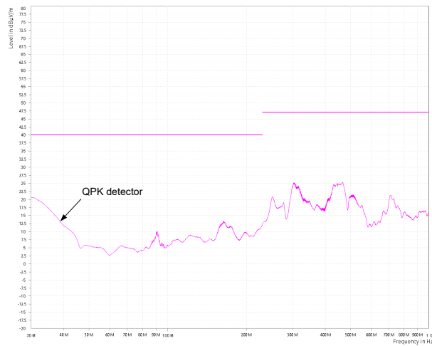
Figure 9-10. CISPR 32 Class B Radiated Emissions: Horizontal Polarization
