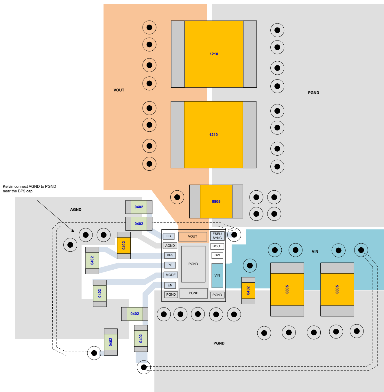
Figure 7-19. Example PCB Layout
