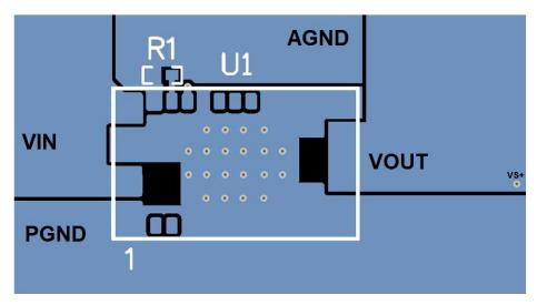
Figure 20. Minimum Component Layout
