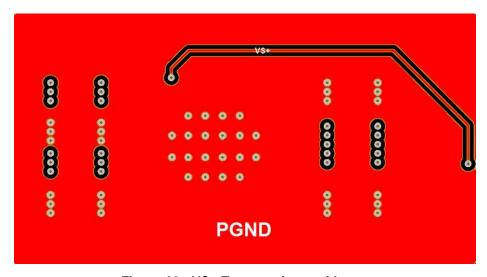
Figure 23. VS+ Trace on Internal Layer
