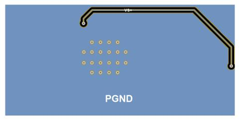
Figure 21. VS+ Trace on Internal Layer
