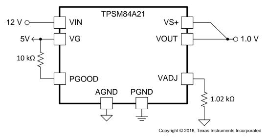
Figure 17. Typical Application Schematic
