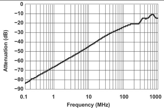
Figure 10. OFF Isolation vs Crosstalk ( $V_+ = 5\text{ V}$ )
