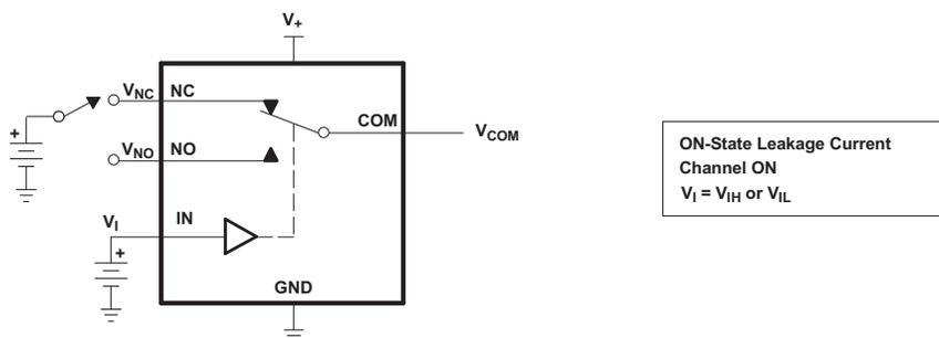
Figure 15. ON-State Leakage Current ( $I_{COM(ON)}$ ,  $I_{NC(ON)}$ ,  $I_{NO(ON)}$ )
