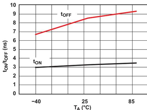
Figure 25.  $t_{ON}$  and  $t_{OFF}$  vs Temperature ( $V_+ = 5$  V)
