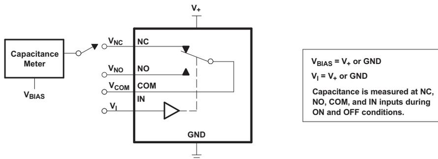
Figure 16. Capacitance ( $C_I$ ,  $C_{COM(ON)}$ ,  $C_{NC(OFF)}$ ,  $C_{NO(OFF)}$ ,  $C_{NC(ON)}$ ,  $C_{NO(ON)}$ )
