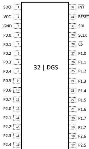
**Figure 4-1. TXE8124 DGS (VSSOP) Package, 32-Pin (Top View)**
