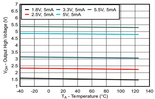
Figure 5-12. I/O High Voltage vs Temperature - 5mA
