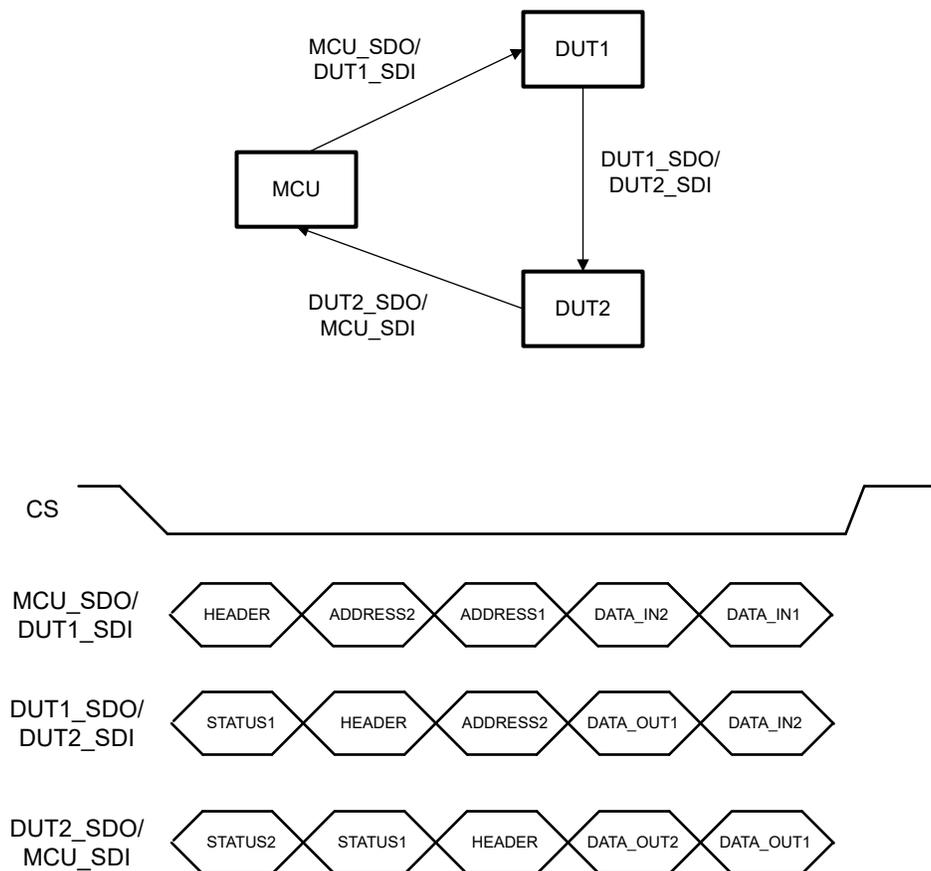
**Figure 7-4. SPI Daisy Chain Diagram**
