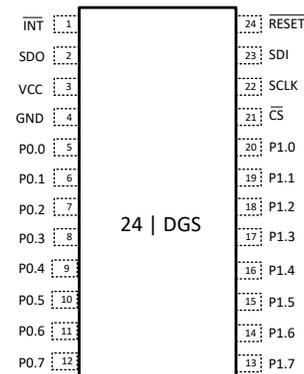
**Figure 4-2. TXE8116 DGS (VSSOP) Package, 24-Pin (Top View)**
