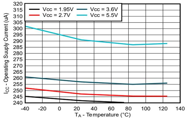
**Figure 5-2. Operating Supply Current vs Temperature ( $f_{SCLK} = 10\text{MHz}$ )**
