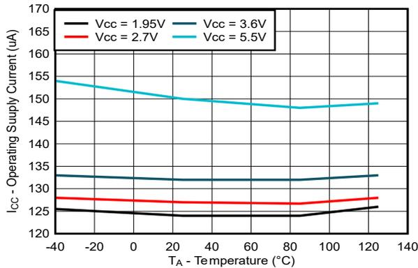
**Figure 5-1. Operating Supply Current vs Temperature ( $f_{SCLK} = 5\text{MHz}$ )**
