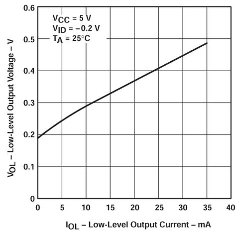
Figure 5-4. Low-level Output Voltage vs Low-level Output Current
