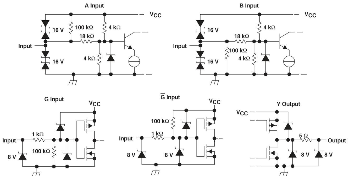
**Figure 7-1. Equivalent Input and Output Schematic Diagrams**
