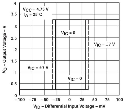
Figure 5-1. Output Voltage vs Differential Input Voltage
