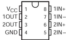
**Figure 4-1. D (SOIC) or P (PDIP) Package
