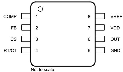
Figure 5-2. DGK Package, 8-Pin VSSOP (Top View)
