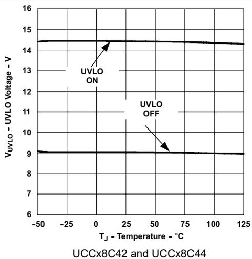
**Figure 6-9. Undervoltage Lockout vs Temperature**
