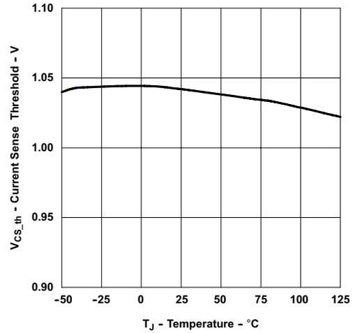
**Figure 6-18. Current Sense Threshold Voltage vs Temperature**
