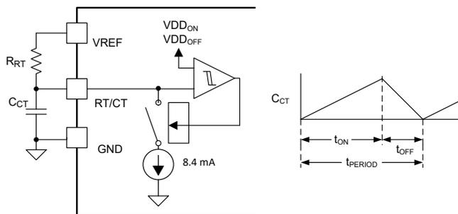
**Figure 7-4. Oscillator Circuit**
