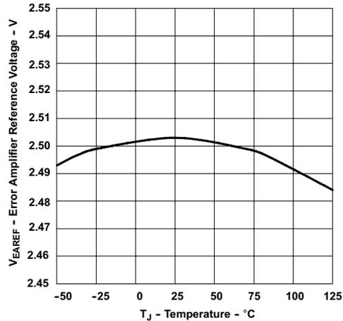
**Figure 6-6. Error Amplifier Reference Voltage vs Temperature**
