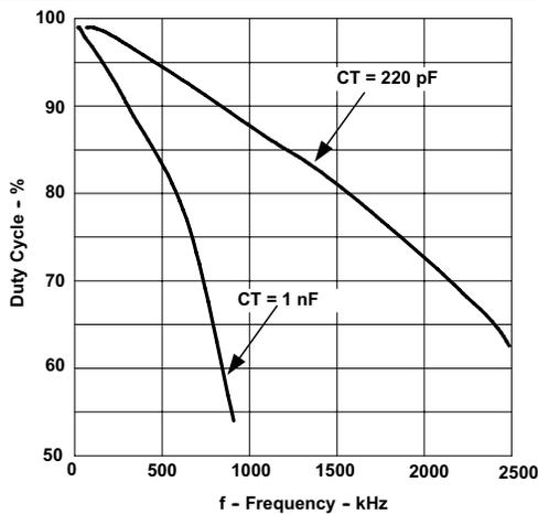
**Figure 6-15. Maximum Duty Cycle vs Oscillator Frequency**
