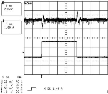
CH1: Output Voltage AC Coupled, 200mV/div
