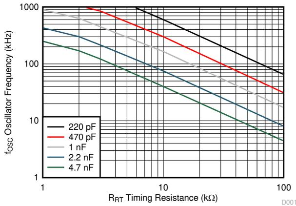
**Figure 6-1. Oscillator Frequency vs Timing Resistance and Capacitance**
