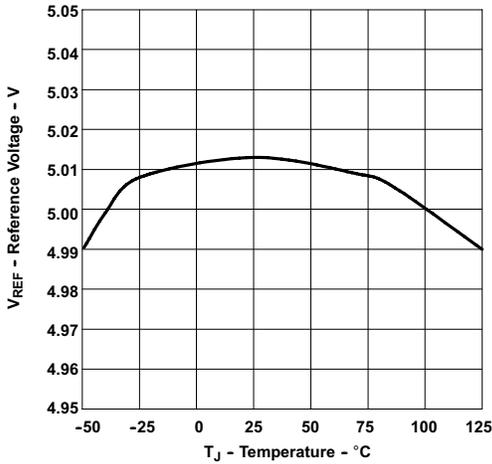
**Figure 6-5. Reference Voltage vs Temperature**
