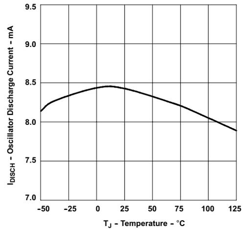
**Figure 6-2. Oscillator Discharge Current vs Temperature**
