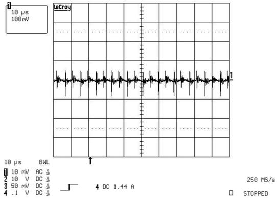
**Figure 8-11. Output Voltage Ripple at Full Load (100mV/div)**
