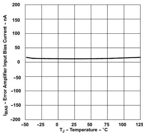
**Figure 6-8. Error Amplifier Input Bias Current vs Temperature**
