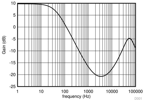
**Figure 8-4. Converter Open-Loop Bode Plot - Gain**
