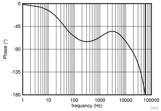
**Figure 8-5. Converter Open-Loop Bode Plot - Phase**
