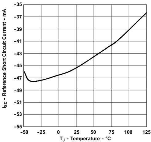
**Figure 6-7. Reference Short-Circuit Current vs Temperature**
