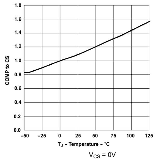
**Figure 6-4. COMP to CS Offset Voltage vs Temperature**
