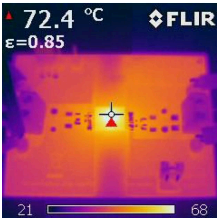
Figure 8-8. UCC33421-Q1 Thermal Image: VINP = 5.0V, VCC = 5.0V, P Out =1.5W
