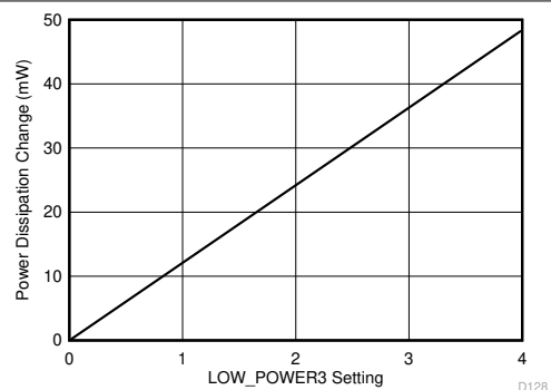
Figure 6-13. Power Dissipation Change vs LOW_POWER3 register setting
