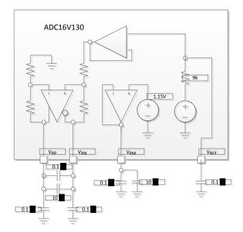
Figure 29. Internal References and their Decoupling
