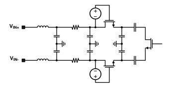
Figure 23. Input Equivalent Circuit
