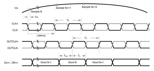
Figure 2. Digital Output Timing
