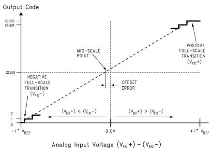
Figure 3. Transfer Characteristic (Offset Binary Format)
