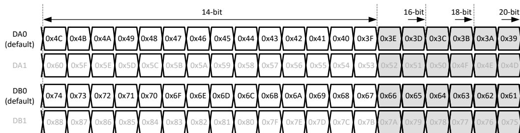
Figure 7-38. 1-wire output bit mapping
