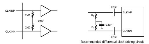
Figure 63. Recommended Differential Clock Driving Circuit
