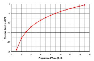
Figure 51. OVR Detection Threshold
