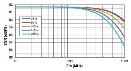
Figure 64. SNR vs Input Frequency and External Clock Jitter
