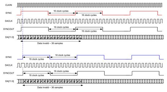
Figure 45. Multiple Device Synchronization Timing Diagram
