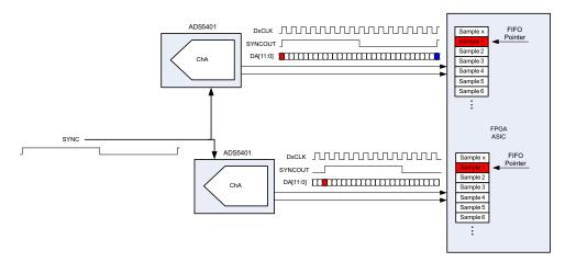
Figure 44. Multiple ADC Synchronization
