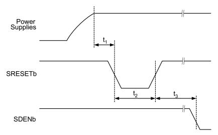
Figure 2. Device Initialization Timing Diagram
