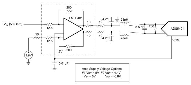
Figure 62. DC-Coupled Single-Ended to Differential Amplifier with 1st Nyquist Lowpass Filter
