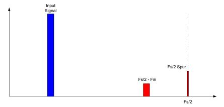
Figure 40. Interleaving Spur at Fs/2 due to Offset Mismatch
