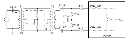
Figure 61. Input Drive Circuit
