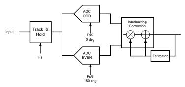
Figure 39. Interleaving Correction Circuit
