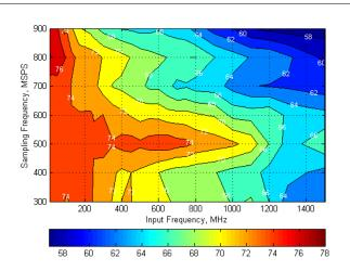
Figure 33. SFDR Across Input and Sampling Frequencies (Auto Off)
