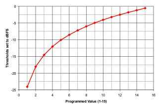
Figure 38. OVR Detection Threshold
