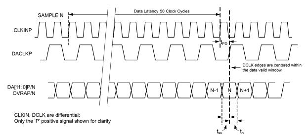
Figure 1. Timing Diagram for 12-Bit DDR Output
