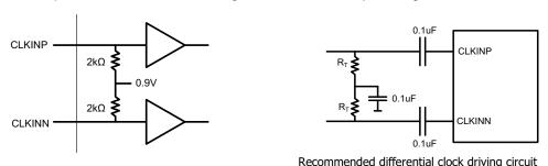
Figure 36. Recommended Differential Clock Driving Circuit
