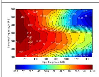
Figure 34. SNR Across Input and Sampling Frequencies (Auto On)
