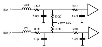
Figure 37. Equivalent Analog Input Circuit
