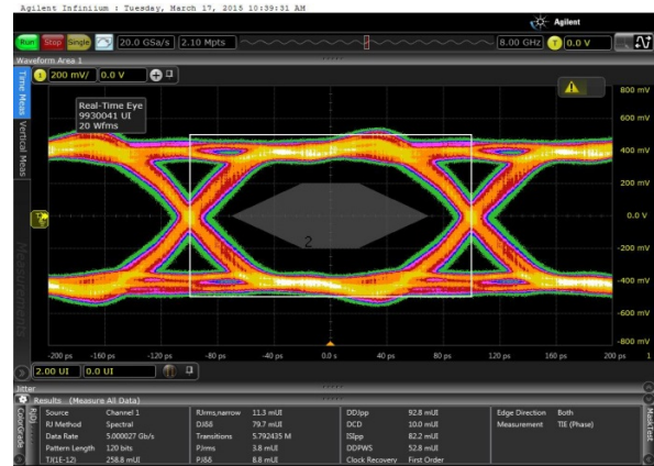
Figure 87. Eye at 5-Gbps Bit Rate with Increased Output Swing
