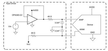
Only one ADC channel is shown in this diagram. Replicate the same circuit for other ADC channels.
