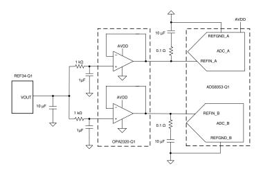
Figure 8-3. Reference Drive Circuit
