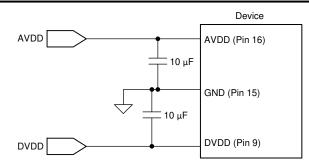
Figure 8-5. Power-Supply Decoupling
