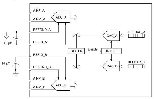
Figure 7-1. Reference Configurations and Connections
