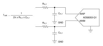
Figure 8-1. Charge Kickback Filter
