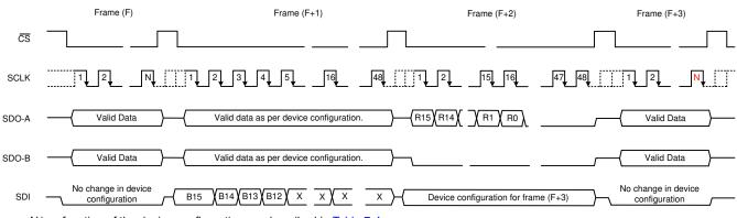
N is a function of the device configuration, as described in Table 7-4.
