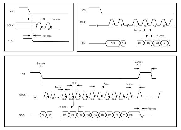
Figure 6-1. Serial Interface Timing Diagram
