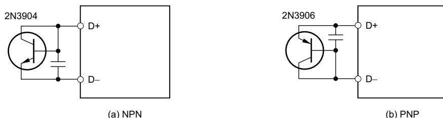
Figure 7-6. Remote Temperature Sensor Using Transistor
