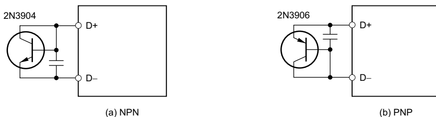
Figure 7-6. Remote Temperature Sensor Using Transistor
