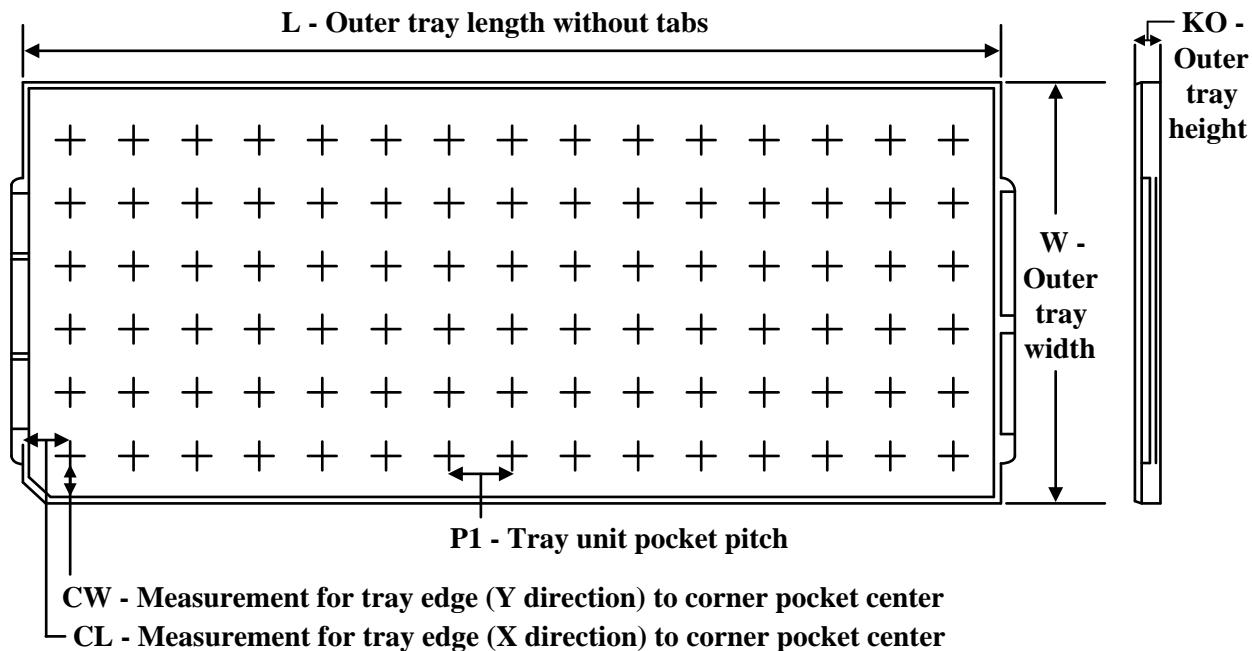
Chamfer on Tray corner indicates Pin 1 orientation of packed units.
