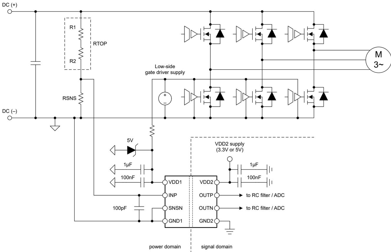
Figure 8-1. Using the AMC0x11D in a Typical Application
