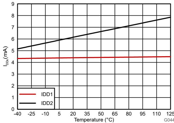
Figure 6-14. Supply Current vs Temperature
