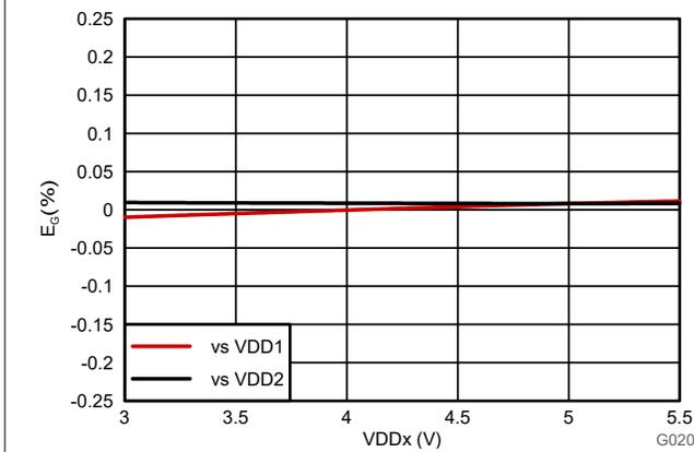
Figure 6-8. Gain Error vs Supply Voltage
