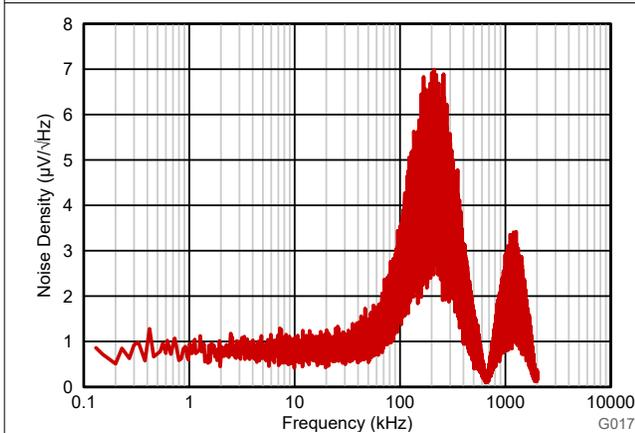
Figure 6-10. Input-Referred Noise Density vs Frequency
