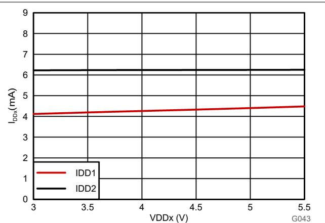
Figure 6-13. Supply Current vs Supply Voltage
