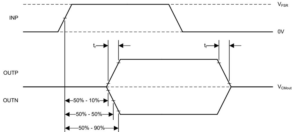
**Figure 6-1. Rise, Fall, and Delay Time Definition**
