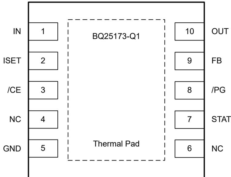
**Figure 5-1. DRC VSON Package 10-Pin (Top View)**
