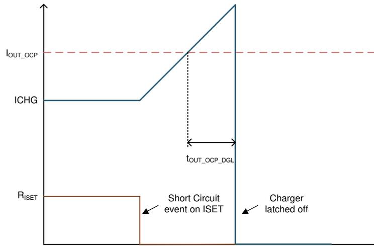
Figure 7-3. Overcurrent Protection
