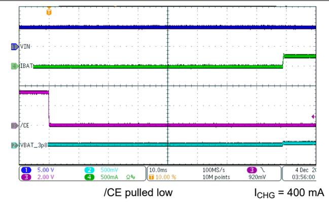
**Figure 8-5. Charge Enable**
