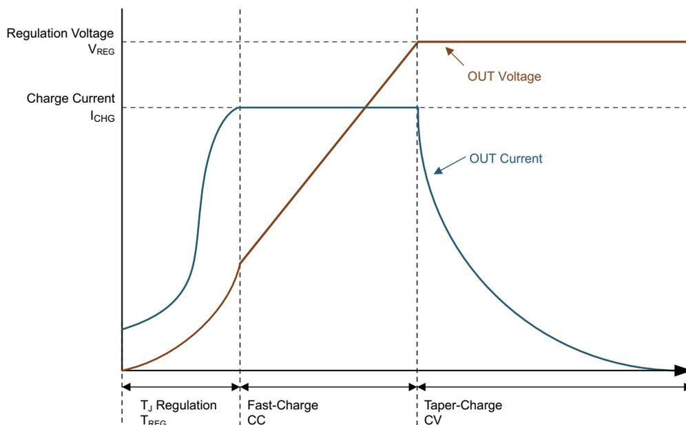
**Figure 7-1. Supercapacitor Charging Profile with Thermal Regulation**
