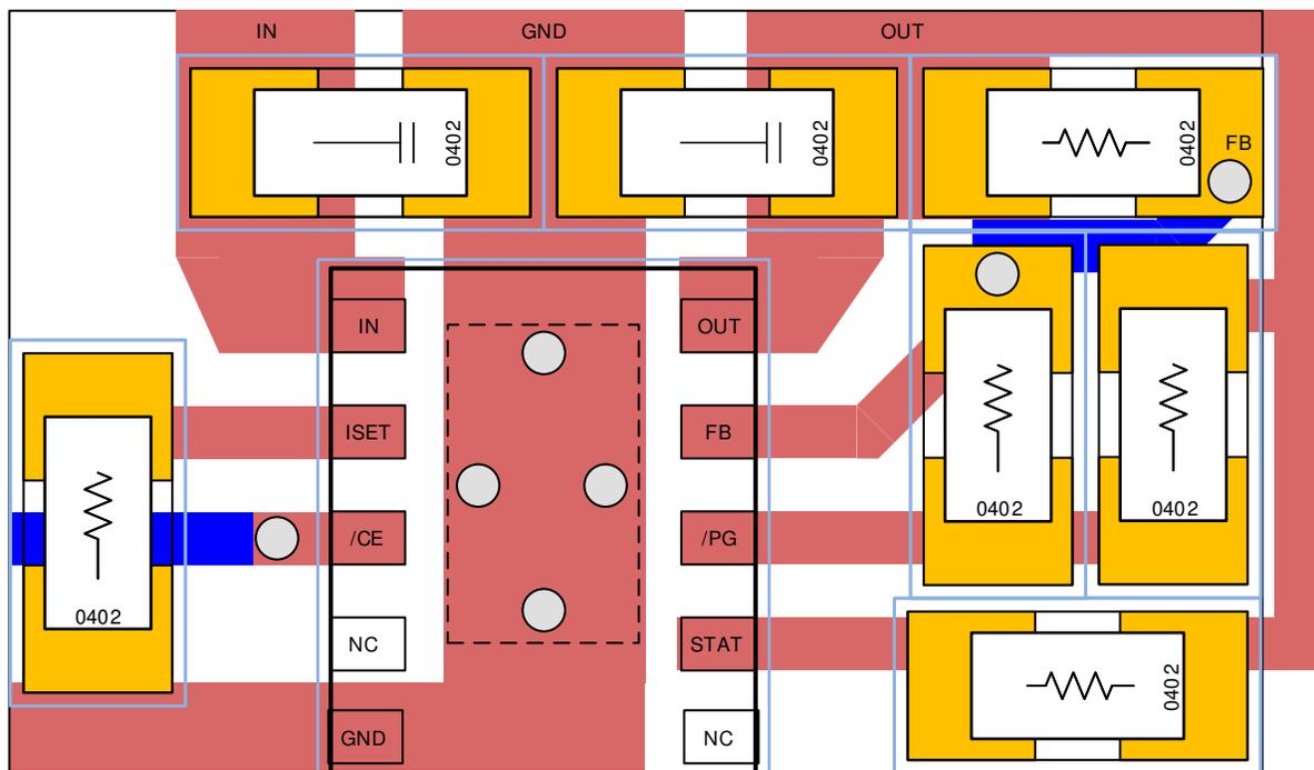
Figure 10-1. BQ25173-Q1 Board Layout Example
