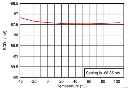
**Figure 7-8. Short Circuit Discharge 1 Protection Threshold vs. Temperature**
