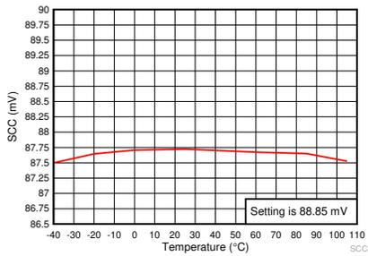
**Figure 7-7. Short Circuit Charge Protection Threshold vs. Temperature**
