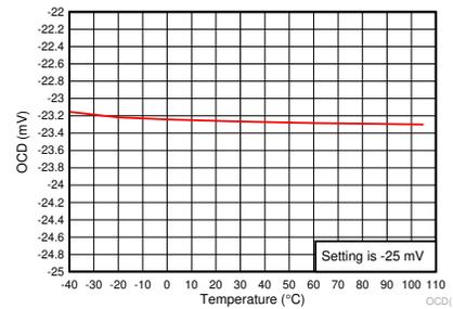
**Figure 7-6. Overcurrent Discharge Protection Threshold vs. Temperature**
