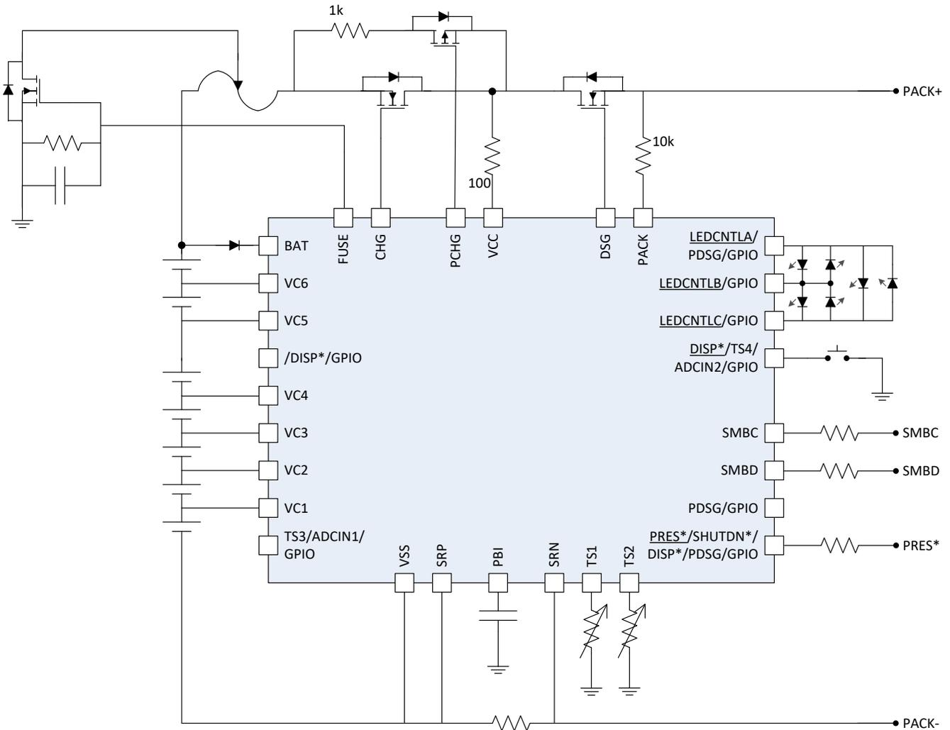
**Figure 8-1. Simplified Schematic of a BQ40Z80 Configuration**
