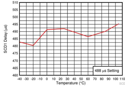
**Figure 7-12. Short Circuit Discharge 1 Delay Time vs. Temperature**
