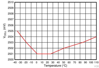
**Figure 7-14. V<sub>CELL</sub> Measurement at 2.5-V vs. Temperature**
