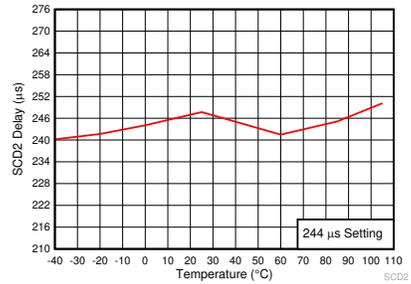
**Figure 7-13. Short Circuit Discharge 2 Delay Time vs. Temperature**
