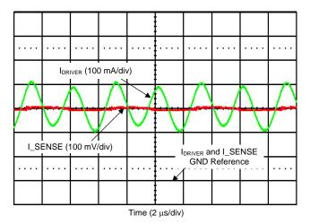
Figure 7. Current-Sense Output in a Wireless Charging Application
