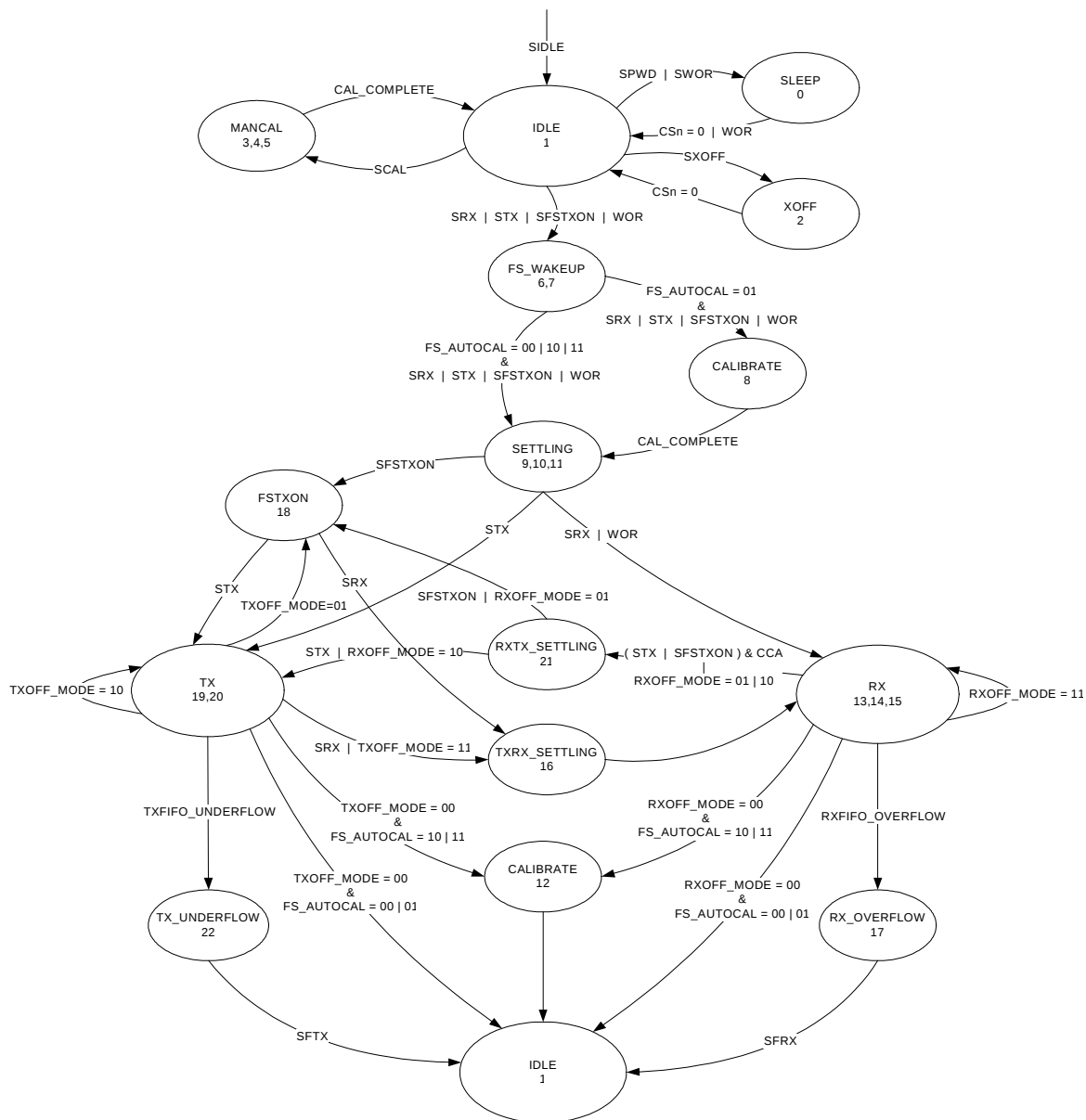
Figure 20: Complete Radio Control State Diagram
