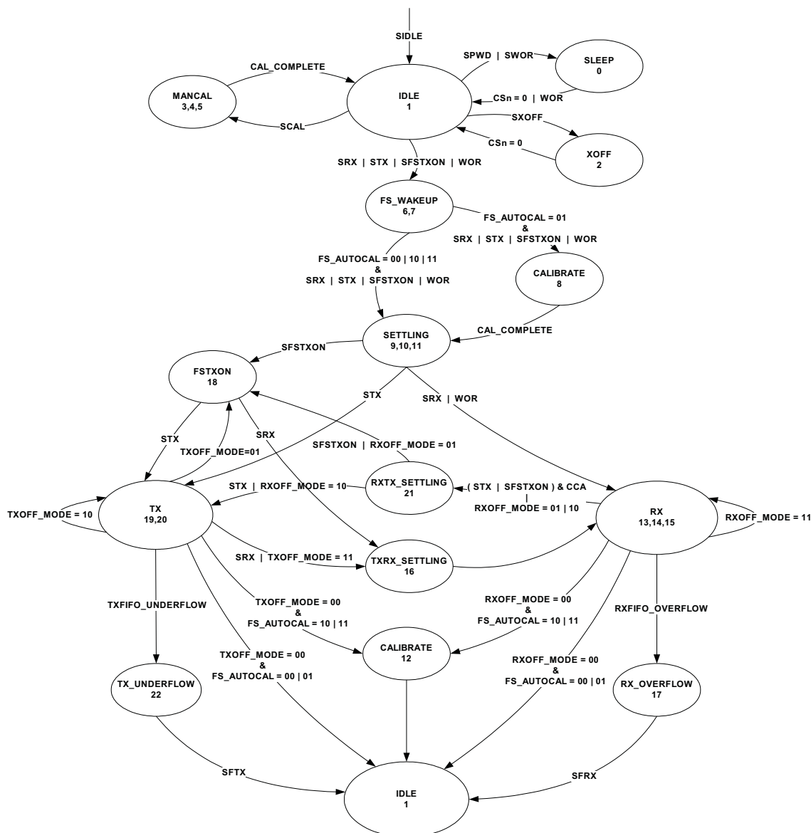
Figure 3-15. Complete Radio-Control State Diagram
