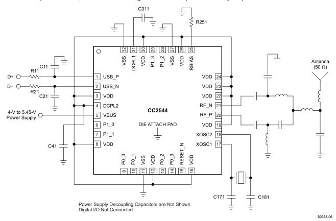
Figure 19. CC2544 Application Circuit
