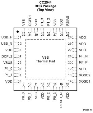
NOTE: The exposed ground pad must be connected to a solid ground plane; this is the main ground connection for the chip.
