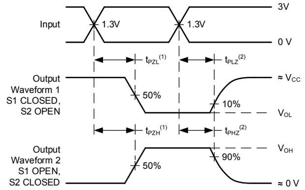
(1)  $t_{PLZ}$  and  $t_{PHZ}$  are the same as  $t_{dis}$ .
