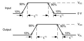
(1) The greater between t<sub>r</sub> and t<sub>f</sub> is the same as t<sub>t</sub>.
