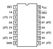
D Package 16-Pin SOIC Top View
