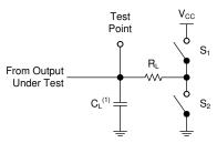
(1) C<sub>L</sub> includes probe and test-fixture capacitance.
