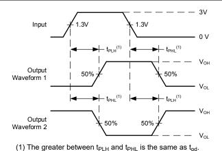
Figure 6-5. Voltage Waveforms, TTL-Compatible CMOS Inputs Propagation Delays
