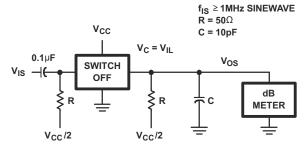
Figure 6-7. Switch OFF Signal Feedthrough
