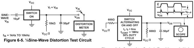
Figure 6-6. Control to Switch Feedthrough Noise Test Circuit
