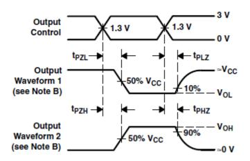
Figure 6-2. Output enable and disable times. Waveform 2
