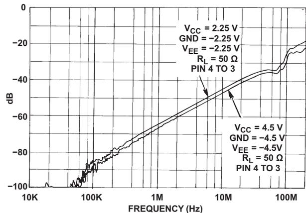
Figure 5-6. Channel OFF Feedthrough (HC and HCT4052)
