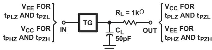
Figure 6-7. Switch ON/OFF Propagation Delay Test Circuit
