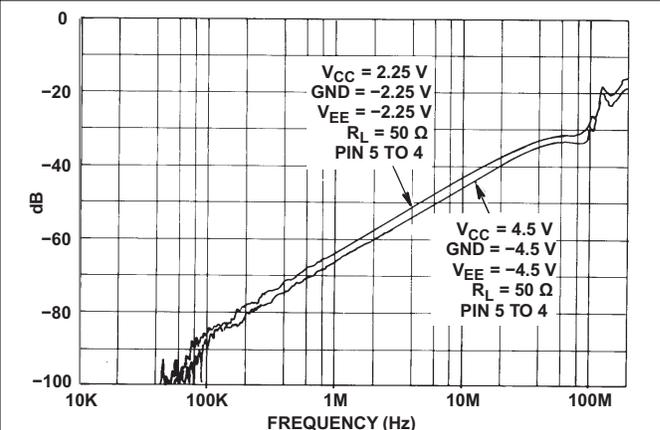
Figure 5-8. Channel OFF Feedthrough (HC and HCT4053)
