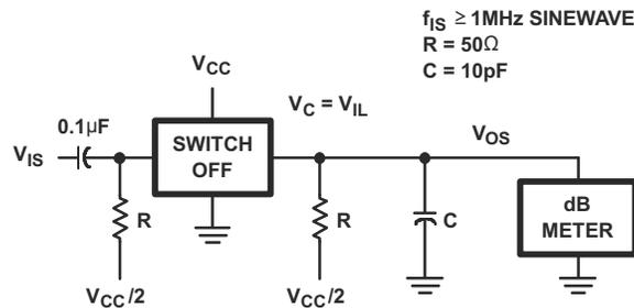
Figure 6-6. Switch OFF Signal Feedthrough
