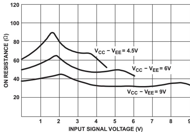
**Figure 8-2. Typical ON Resistance vs Input Signal Voltage**
