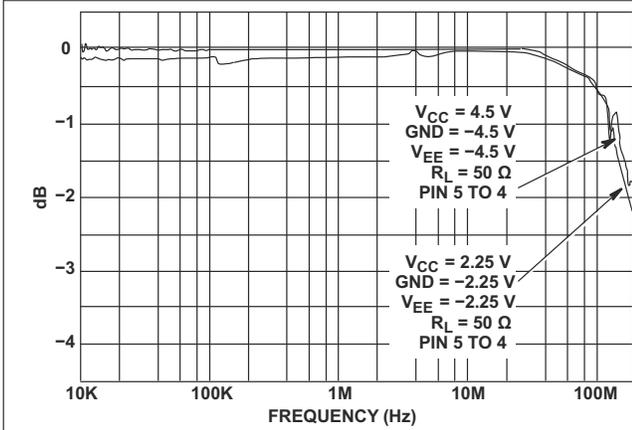
Figure 5-7. Channel ON Bandwidth (HC and HCT4053)
