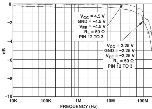
Figure 5-3. Channel ON Bandwidth (HC and HCT4051)
