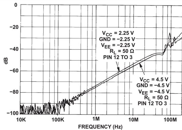
Figure 5-4. Channel OFF Feedthrough (HC and HCT4051)
