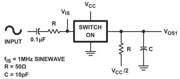
Figure 6-3. Crosstalk Between Two Switches Test Circuit
