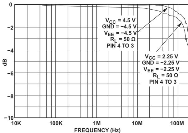
Figure 5-5. Channel ON Bandwidth (HC and HCT4052)
