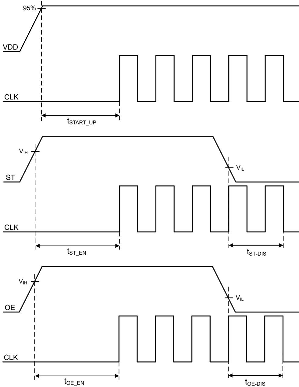
Figure 6-2. Power-On Characteristics
