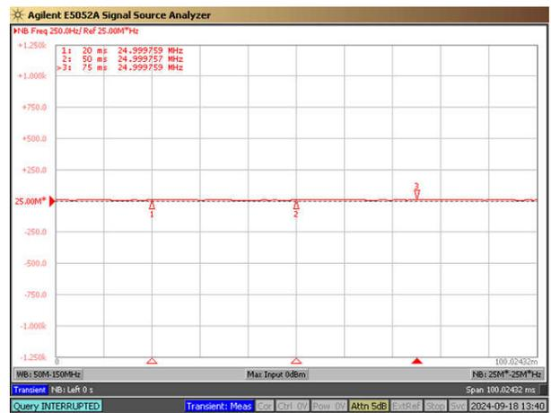
**Figure 8-9. During 1500g Mechanical Shock at 25MHz and 25°C, Y-Axis**
