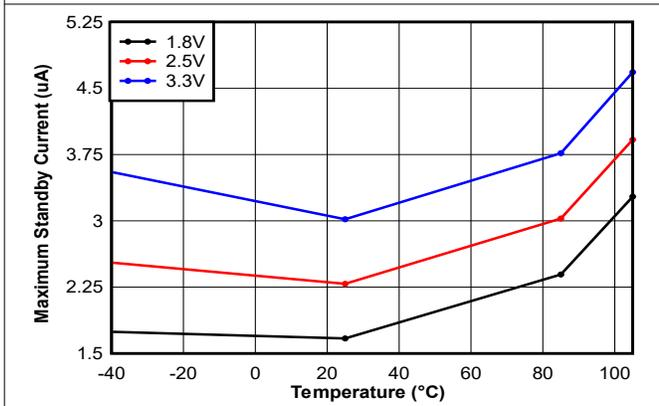
**Figure 6-7. Maximum Standby Current vs Temperature and Supply Voltage**
