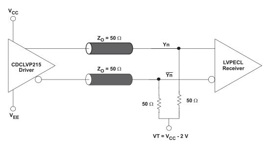
Figure 2. Typical Termination for Output Driver (See the Application Note Interfacing Between LVPECL, LVDS, and CML, Literature Number SCAA056)
