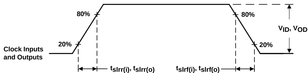
Figure 8. Input and Output Slew Rates
