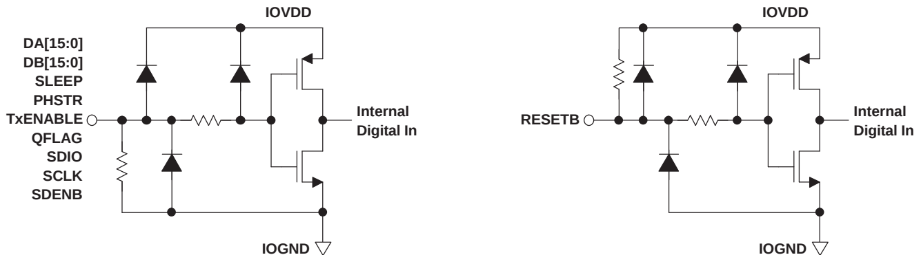
Figure 61. CMOS/TTL Digital Equivalent Input
