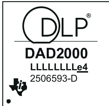
Figure 12-1. Device Marking (Device Top View)
