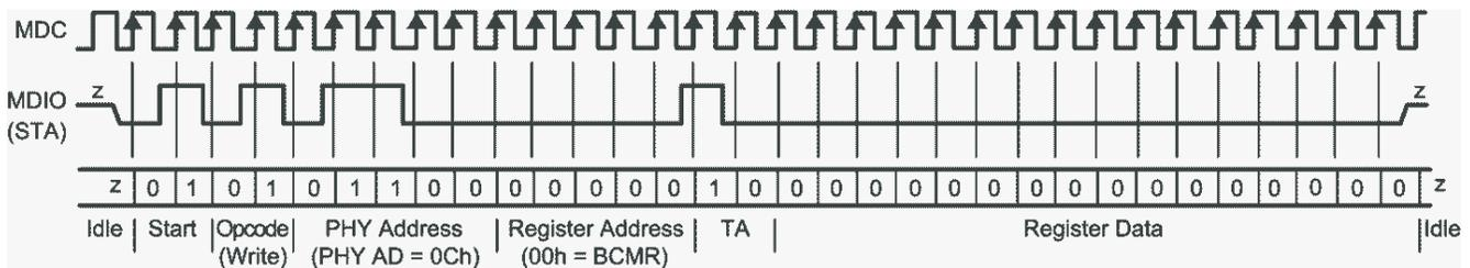
Figure 9-14. Typical MDC/MDIO Write Operation
