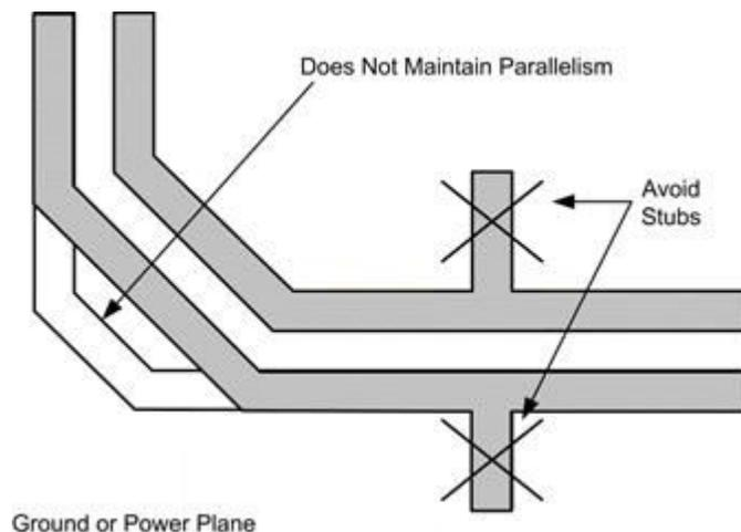
**Figure 12-1. Avoiding Stubs in a Differential Signal Pair**
