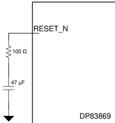
**Figure 9-17. RESET\_N Circuit**
