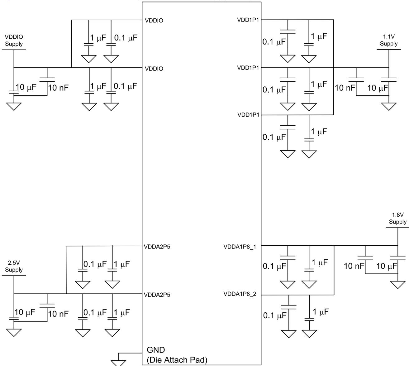
**Figure 11-3. Three-Supply Configuration**
