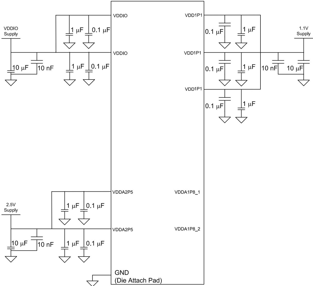
Figure 11-1. Two-Supply Configuration
