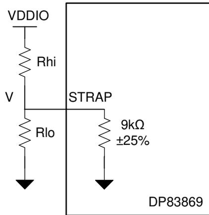
**Figure 9-15. Strap Circuit**
