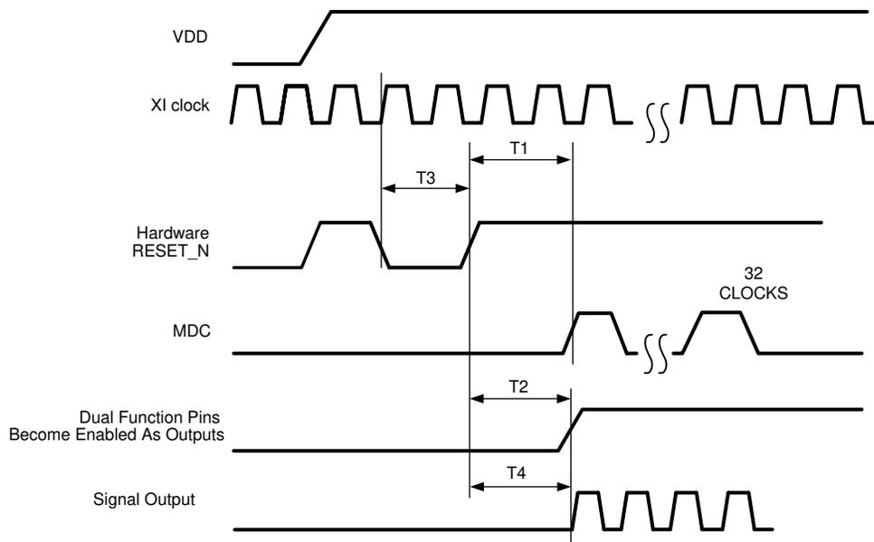
**Figure 8-2. Reset Timing**
