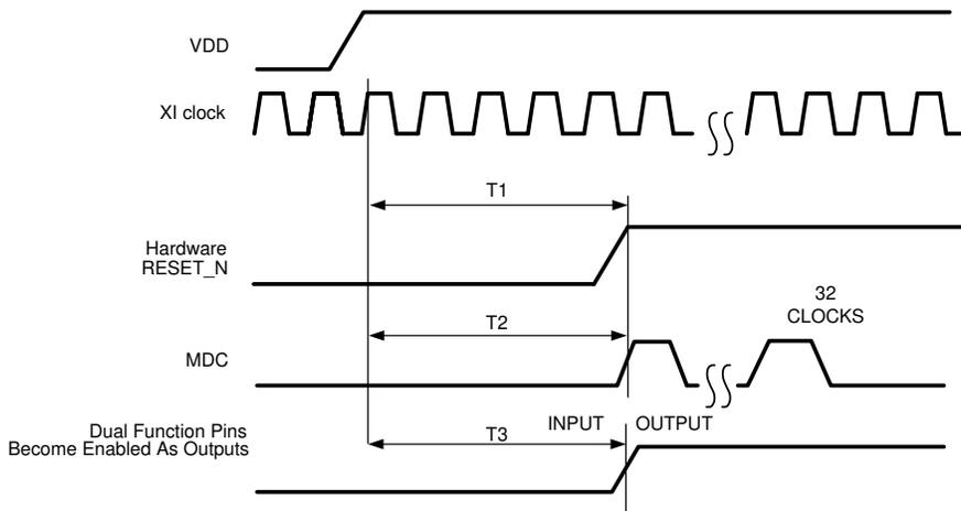
**Figure 8-1. Power-Up Timing**
