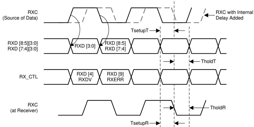
**Figure 8-7. RGMII Receive Multiplexing and Timing Diagram**
