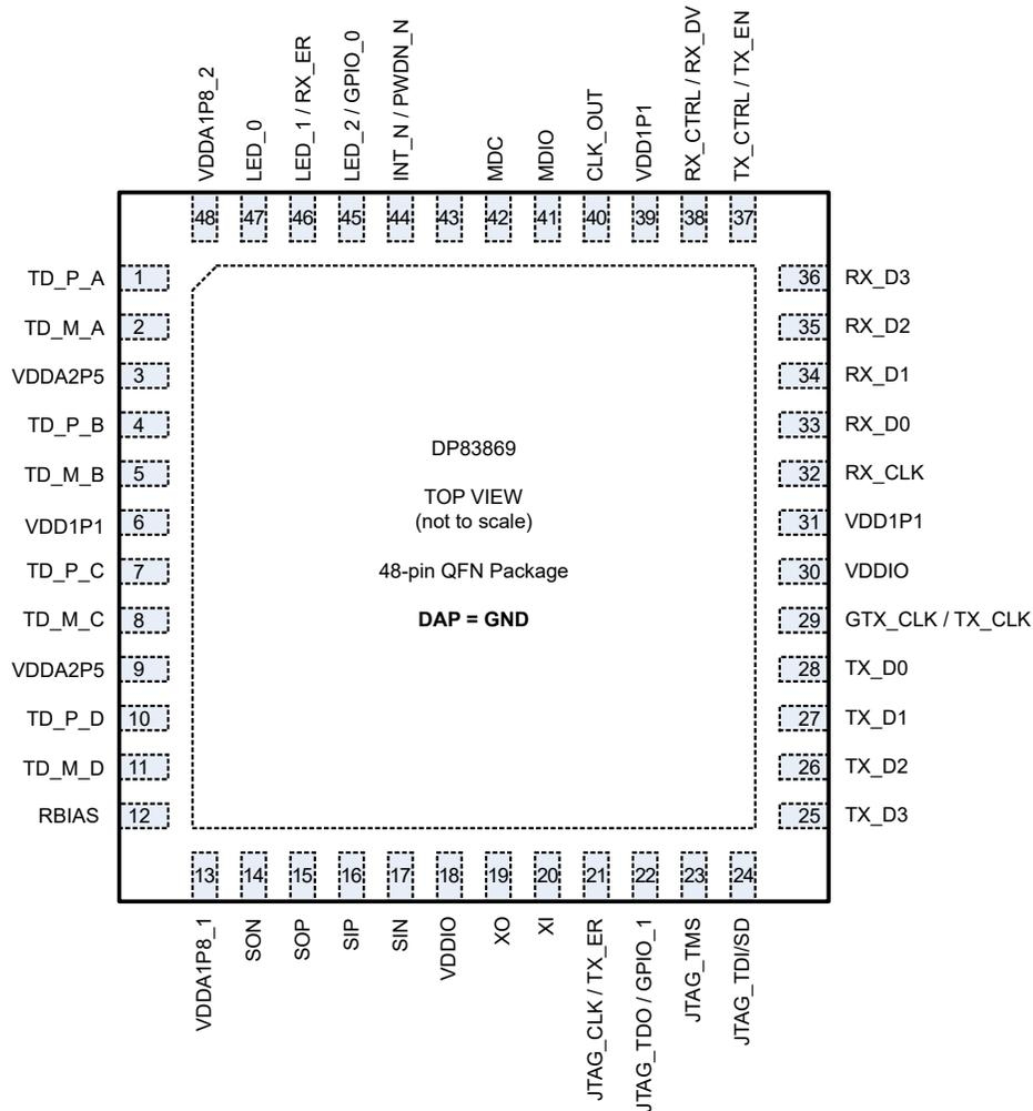
Figure 7-1. RGZ Package (48-Pin VQFN) Top View
