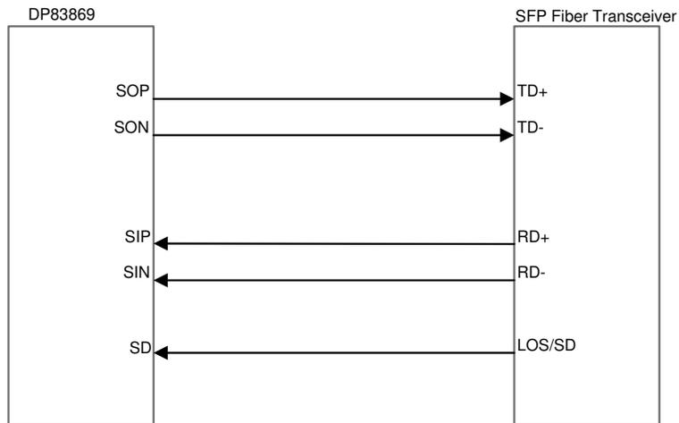
SFP Fiber Transceiver usually have integrated AC coupling capacitors. Adding external capacitors may not be needed.
