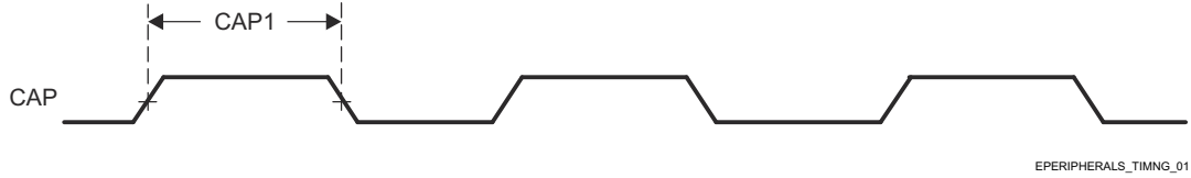
Figure 6-56. eCAP Input Timings
