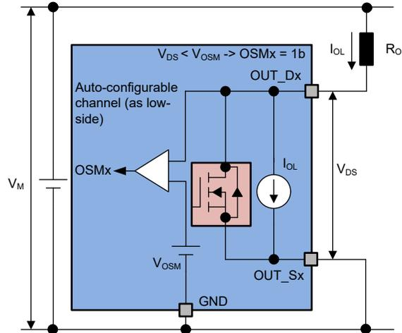
**Figure 7-18. Output Status Monitor - Auto-configurable Channel as Low-side**
