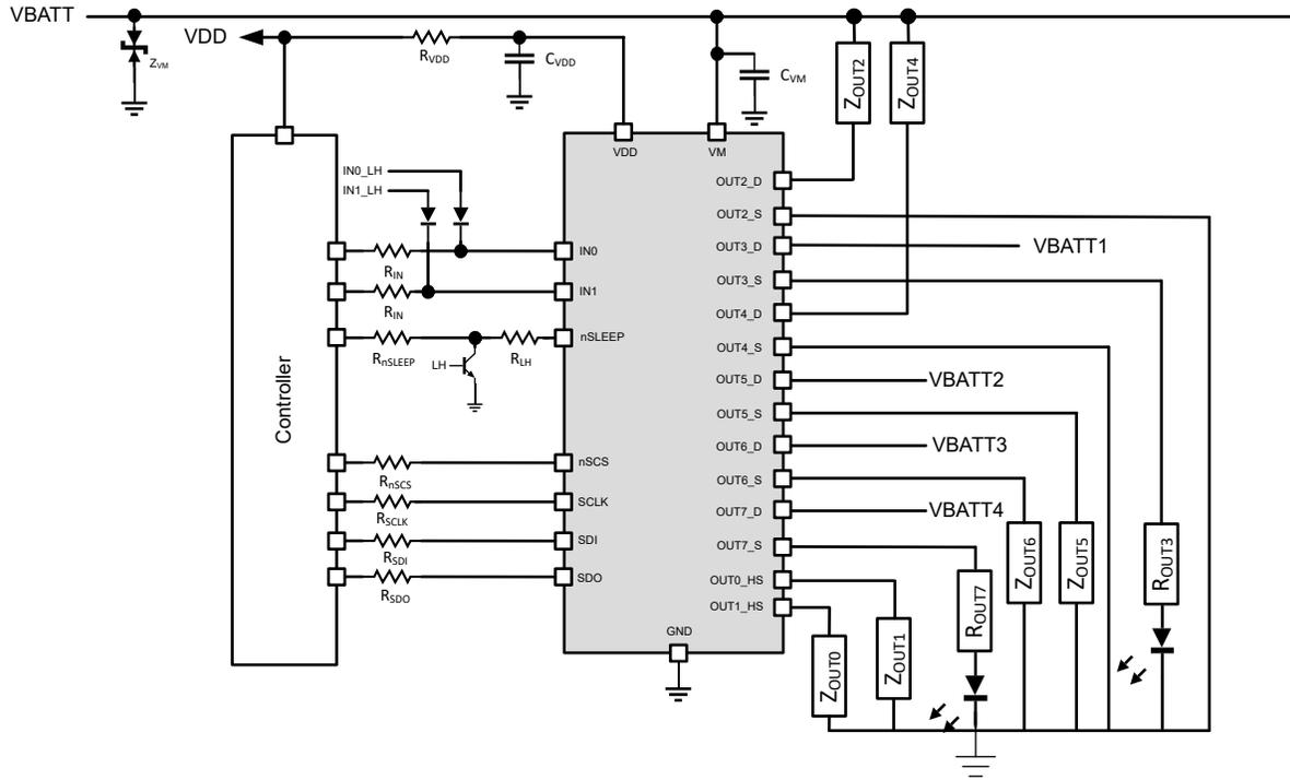
Figure 8-2. Application Schematic
