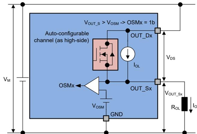
Figure 7-17. Output Status Monitor - Auto-configurable Channel as High-side
