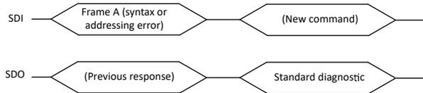
**Figure 7-29. Response After a Command Syntax Error**
