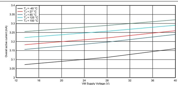
Figure 6-3. Active mode supply current, VDD = 5.5V
