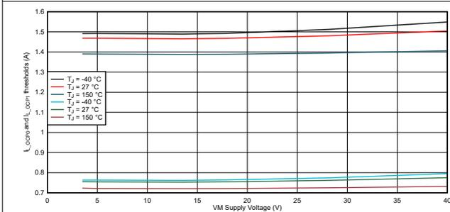
Figure 6-8. Overcurrent Protection Threshold, VDD = 5.5V, OCP = 0b
