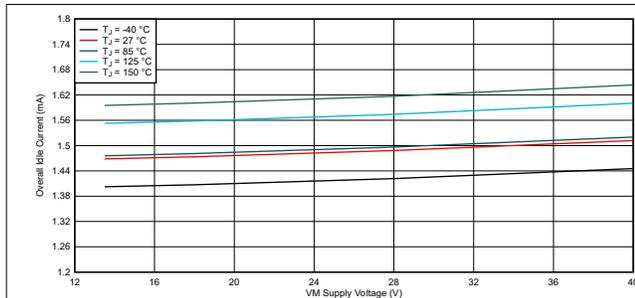
Figure 6-2. Idle mode supply current, VDD = 5.5V
