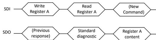
**Figure 7-26. Register content sent back to microcontroller**
