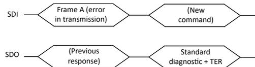
**Figure 7-27. Response After a Error in Transmission**
