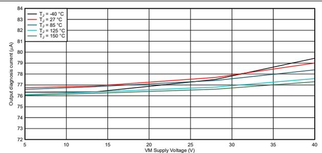
Figure 6-9. Output Diagnosis Current, VDD = 5.5V
