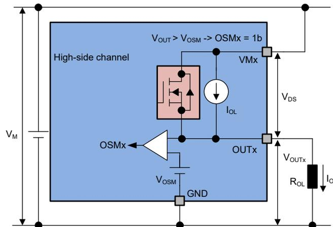
**Figure 7-19. Output Status Monitor - High-side Channels**
